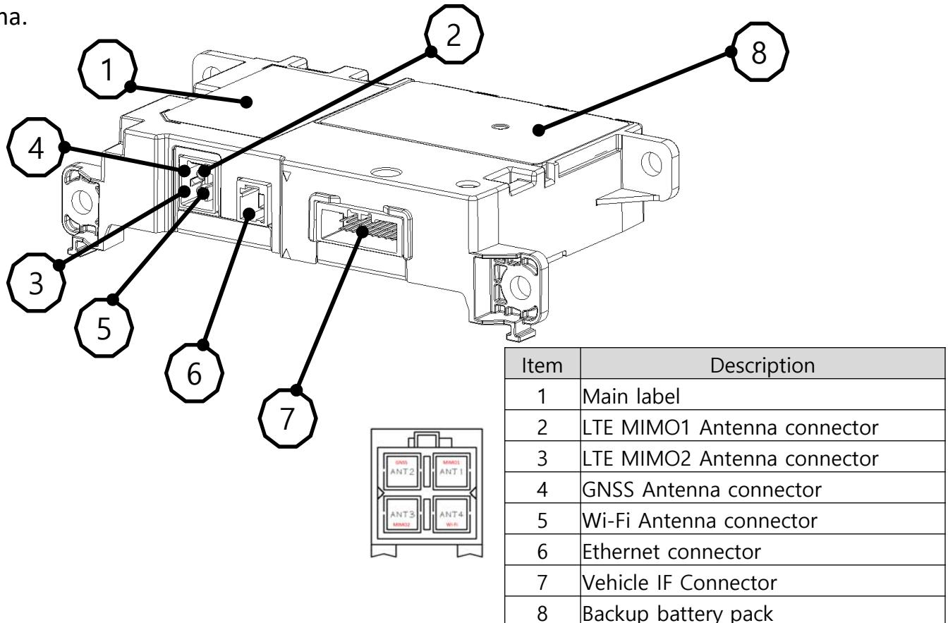
A back-up battery pack, consisting of a battery cell, is integrated into the TCU.
