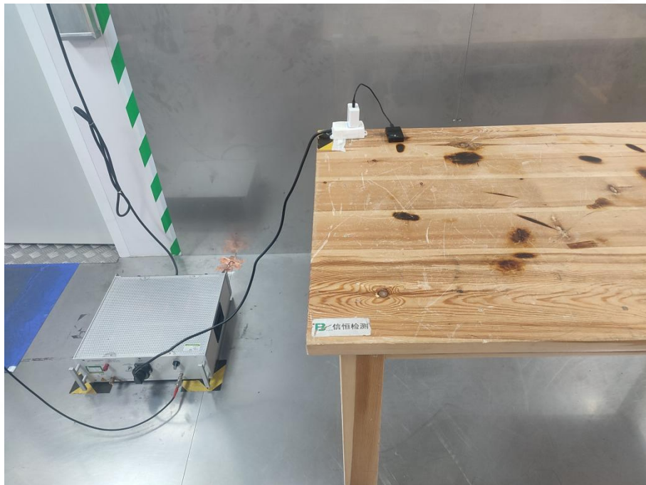
AC Power Line Conducted Emission
