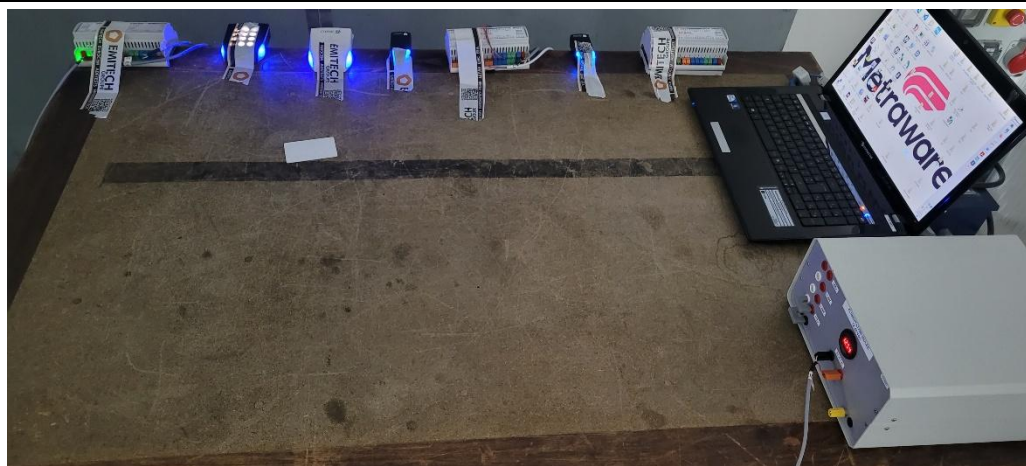
TEST SETUP PHOTO(S) - POWER SUPPLY 120VAc/60Hz / RF OFF
