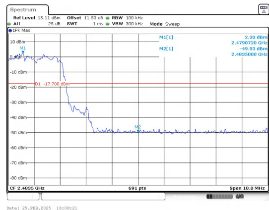
Out Of Band Emission(Right) \pi/4 DQPSK_2-DH5_Channel Hopping
