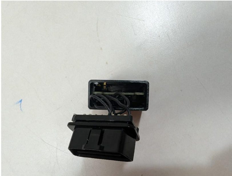
Photograph 12: View of the EUT Placement in Enclosure
