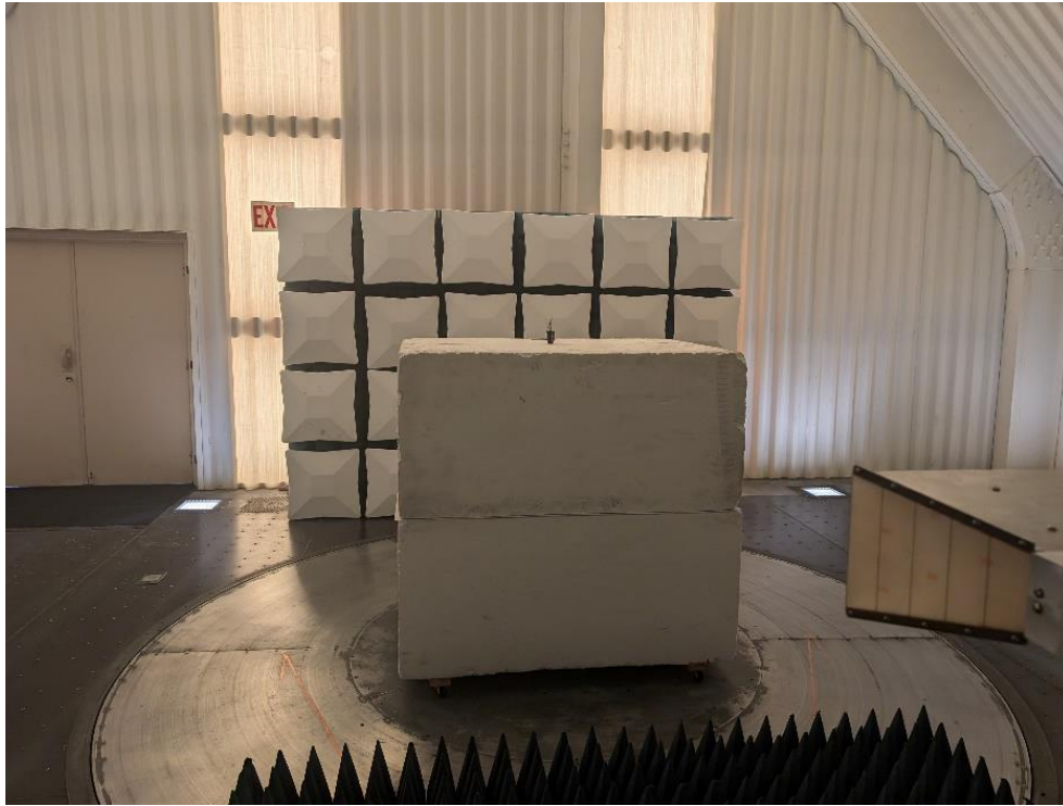
Photograph 3: Front View Radiated Emissions Worst Case – Above 1000 MHz Configuration
