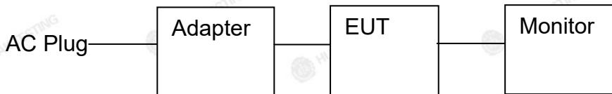
Operation of EUT during above 1GHz radiation testing:
