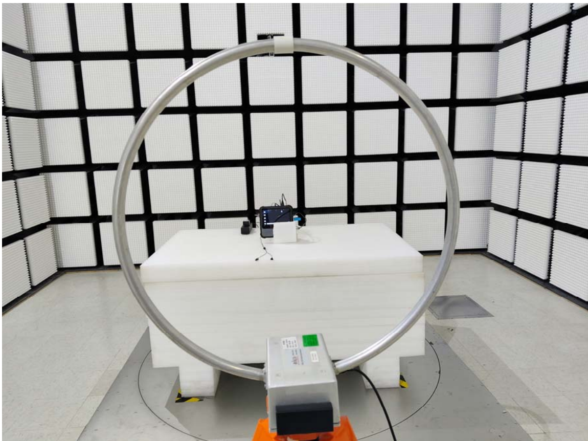
Radiated Emission 9 kHz-30 MHz Parallel View
