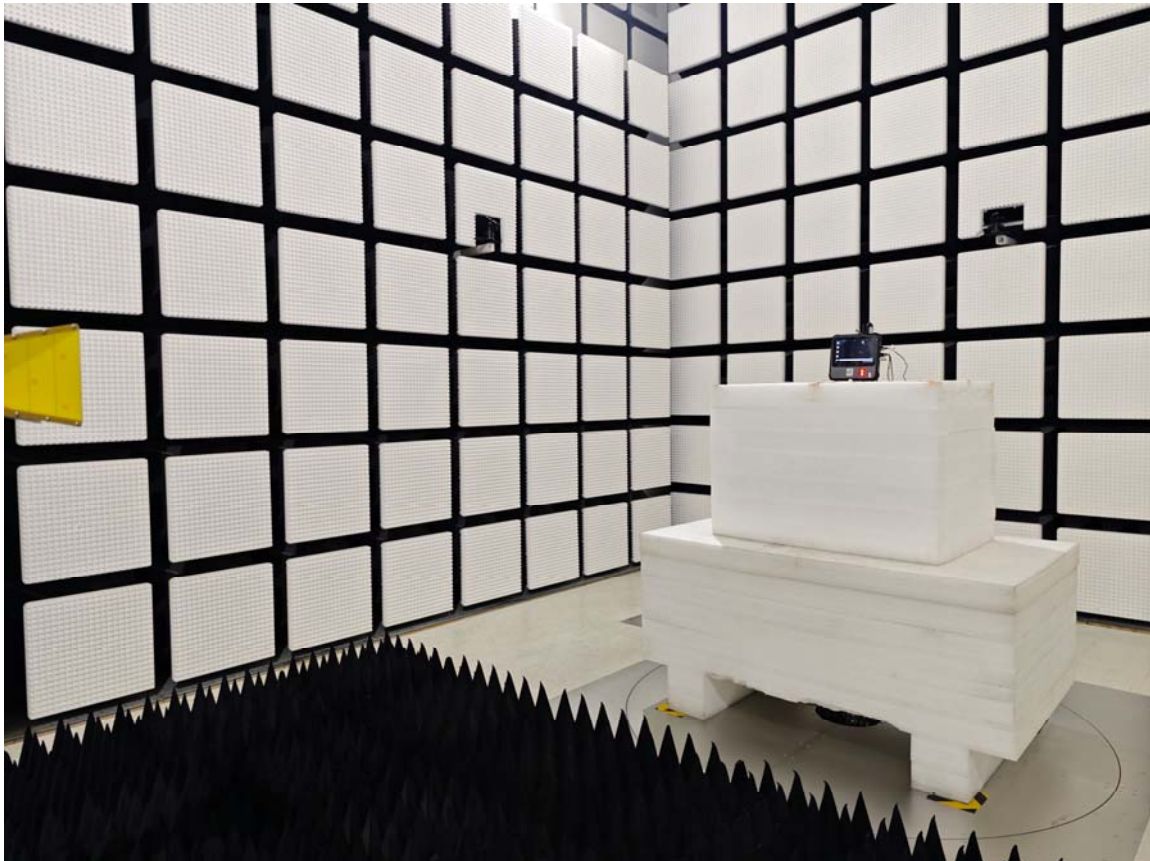
Radiated Emission Above 18-25GHz View
