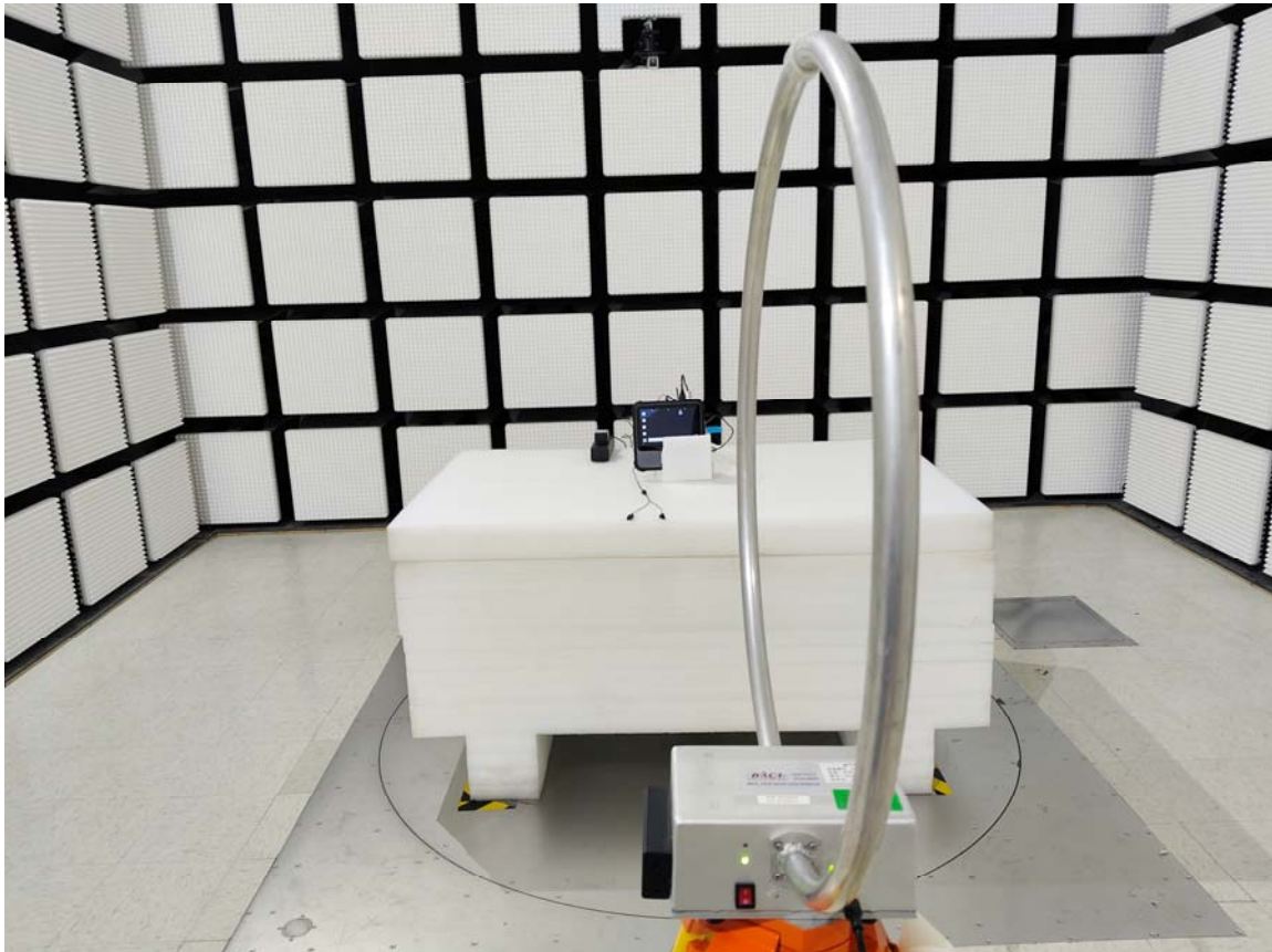
Radiated Emission 9 kHz-30 MHz Ground-parallel View
