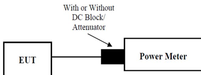
A short RF cable with low cable loss connected to the EUT antenna port. The insert loss of this RF cable/attenuator was offset into the setting of test equipment.
