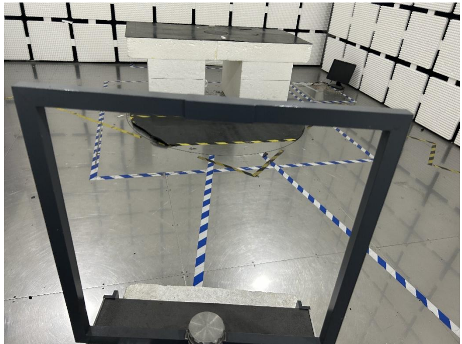
Radiation Emission Test Setup (Below 30MHz)
