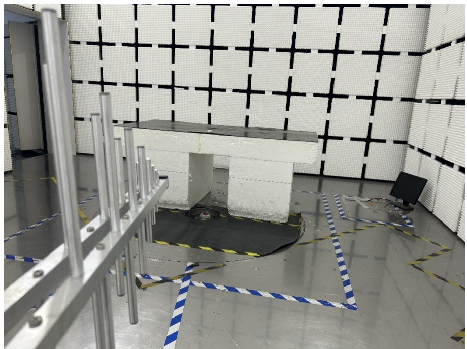
Radiation Emission Test Setup (30MHz to 1GHz)
