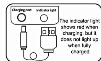
The indicator light shows red when charging, but it does not light up when fully charged
