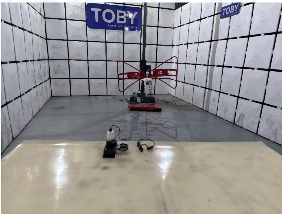
Photo of Setup for Radiated Emission (30MHz~1GHz)
