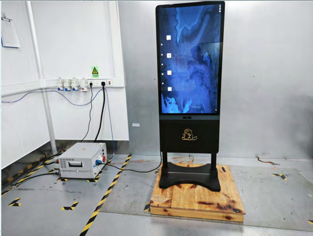
Conducted Emission at AC power line
