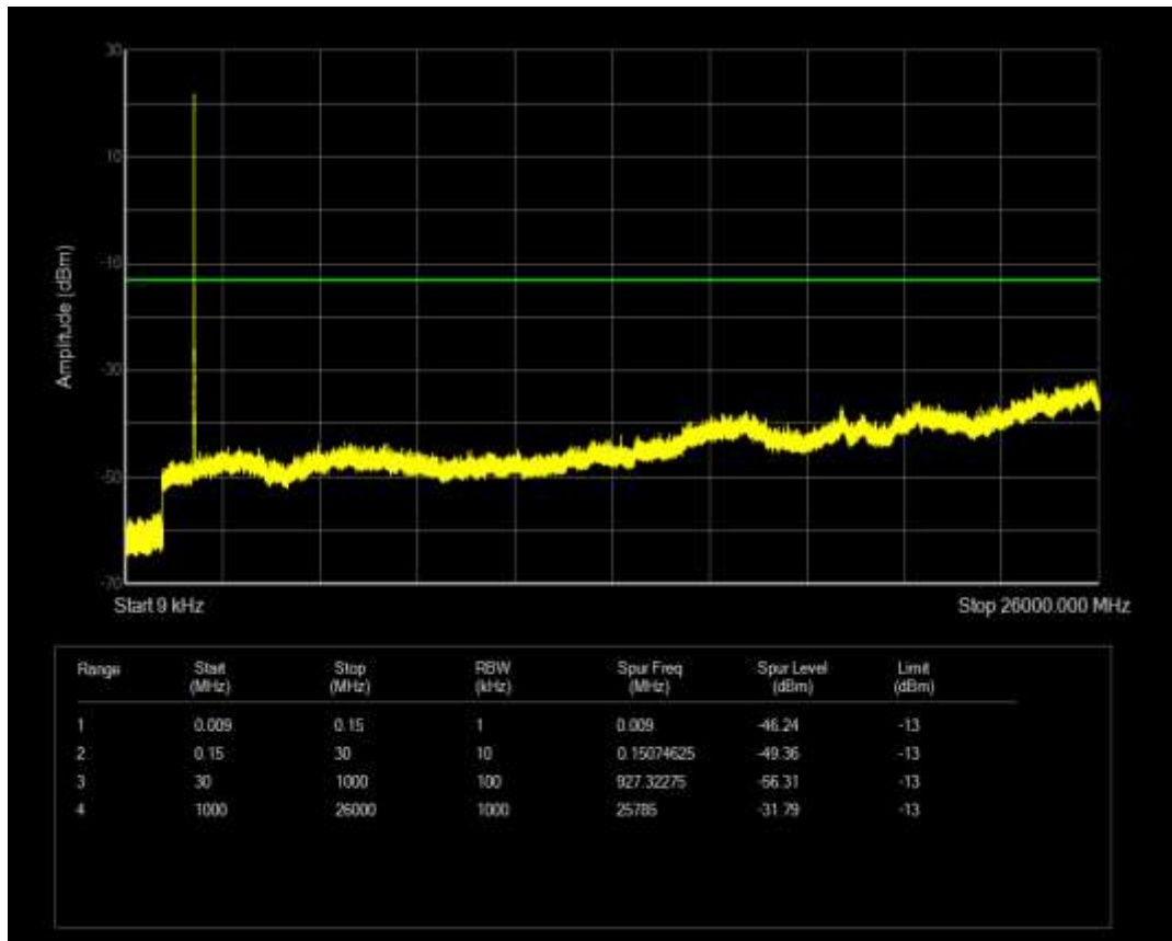
Band2 QAM16 BW=3MHz Channel=19185 RB Size=15 Position=#0
