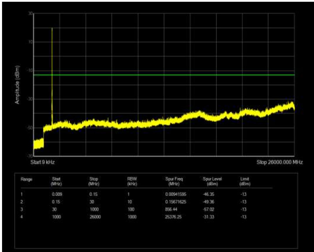
Band2 QAM16 BW=5MHz Channel=19175 RB Size=25 Position=#0
