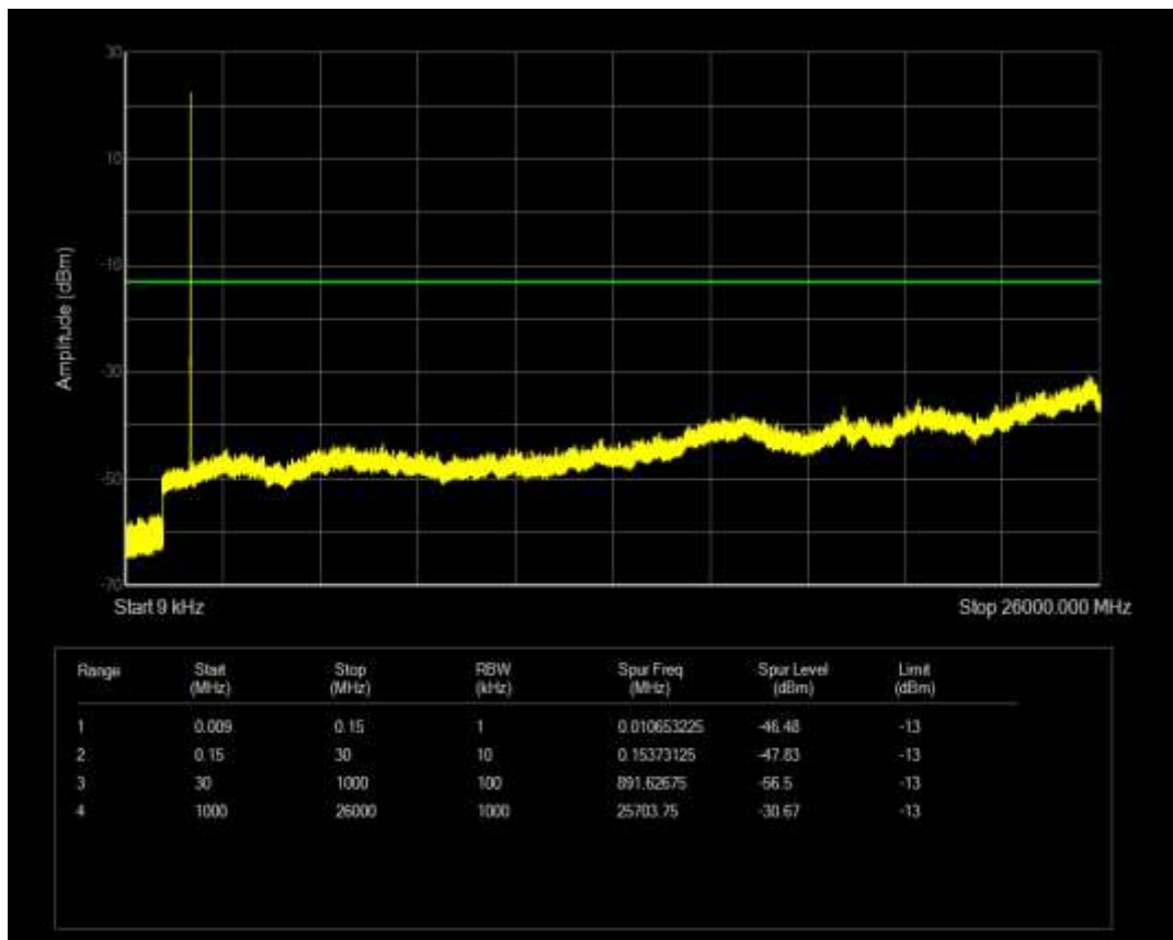
Band4 QPSK BW=3MHz Channel=20385 RB Size=15 Position=#0
