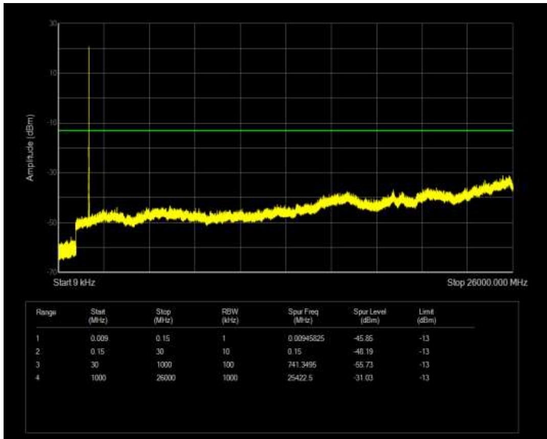
Band4 QAM16 BW=5MHz Channel=19975 RB Size=25 Position=#0
