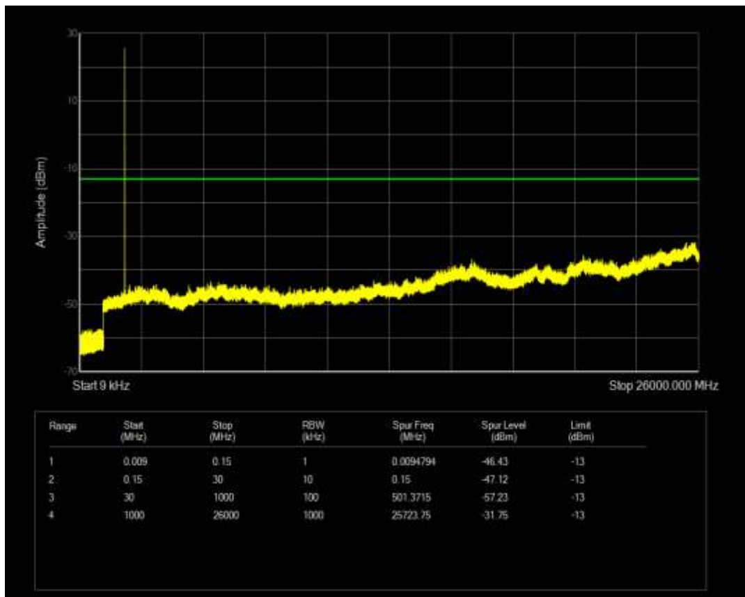
Band2 QPSK BW=1.4MHz Channel=19193 RB Size=6 Position=#0
