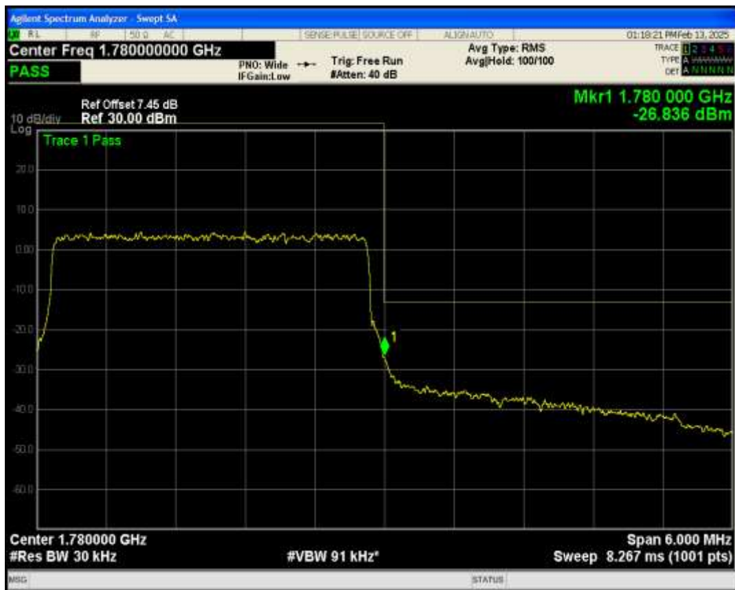
Band66 QAM16 BW=5MHz Channel=131997 RB Size=25 Position=#0
