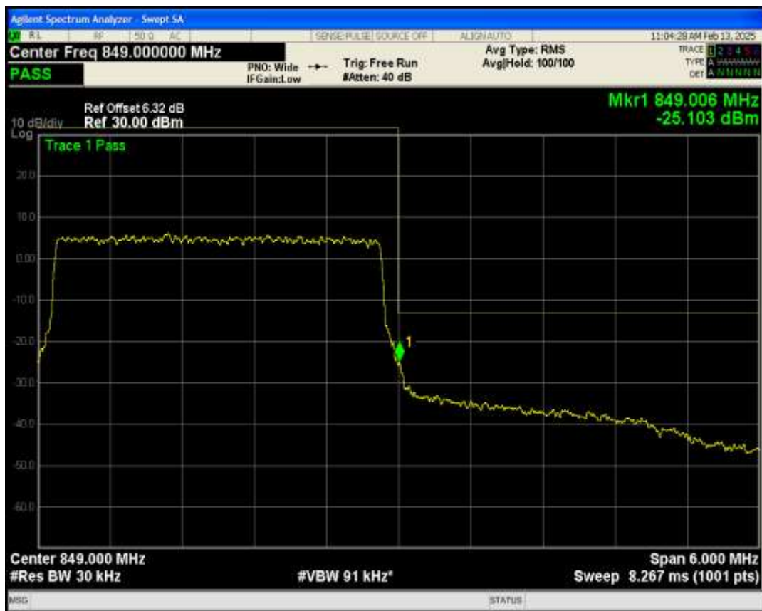
Band5 QAM16 BW=3MHz Channel=20635 RB Size=15 Position=#0
