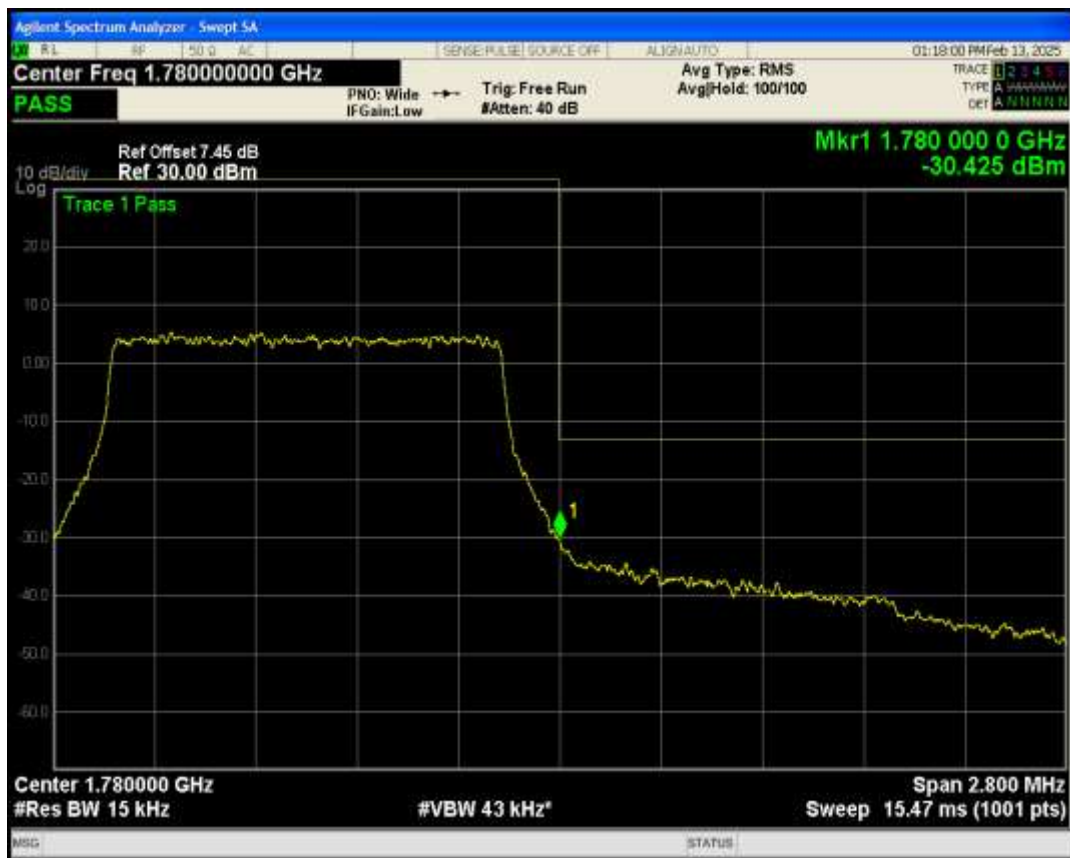
Band66 QAM16 BW=3MHz Channel=131987 RB Size=15 Position=#0
