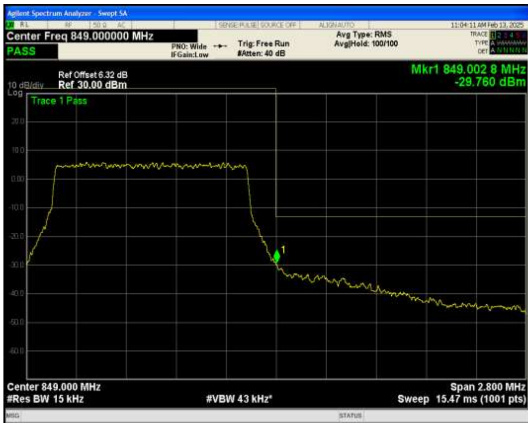
Band5 QAM16 BW=3MHz Channel=20415 RB Size=15 Position=#0
