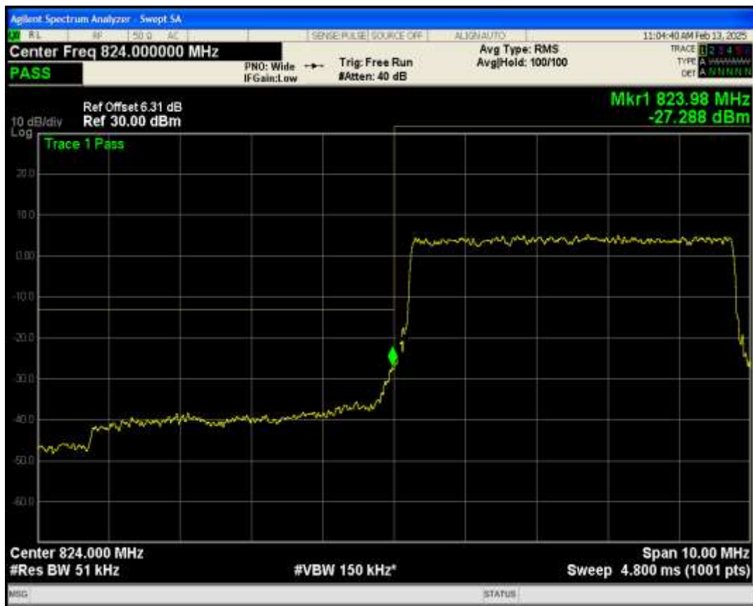
Band5 QPSK BW=5MHz Channel=20625 RB Size=25 Position=#0
