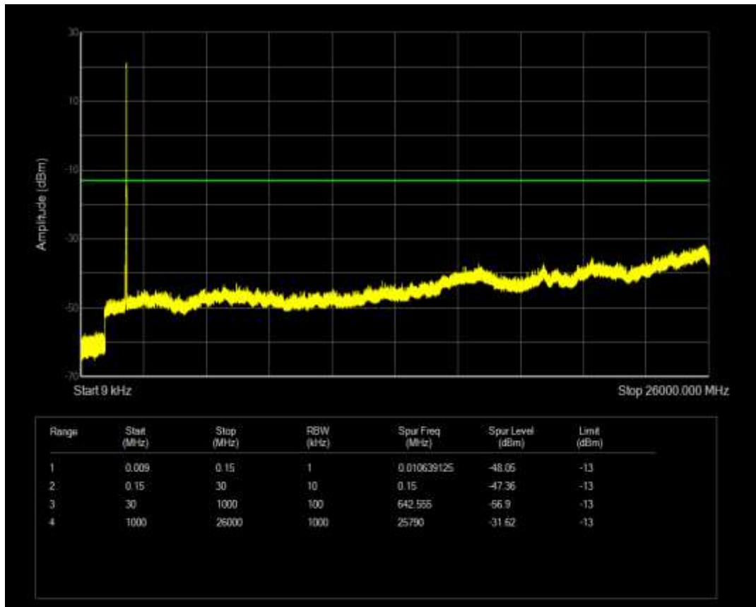
Band2 QPSK BW=15MHz Channel=18675 RB Size=75 Position=#0
