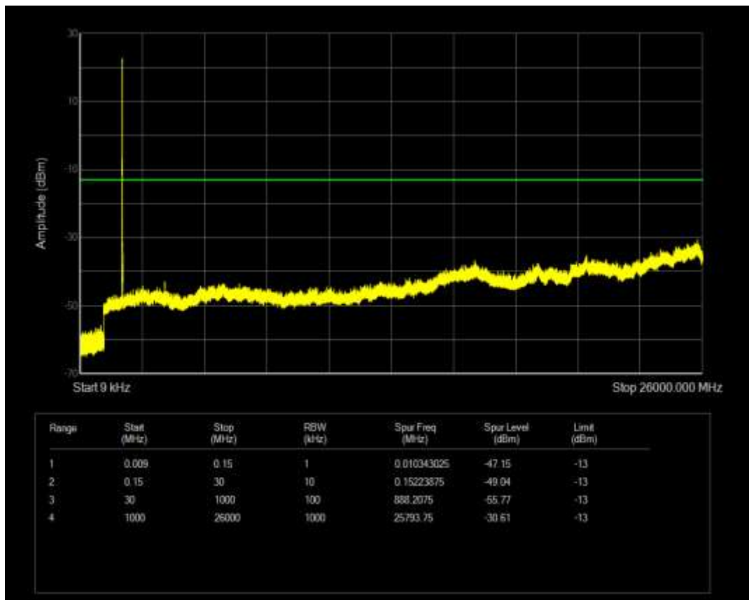
Band66 QAM16 BW=5MHz Channel=132647 RB Size=25 Position=#0
