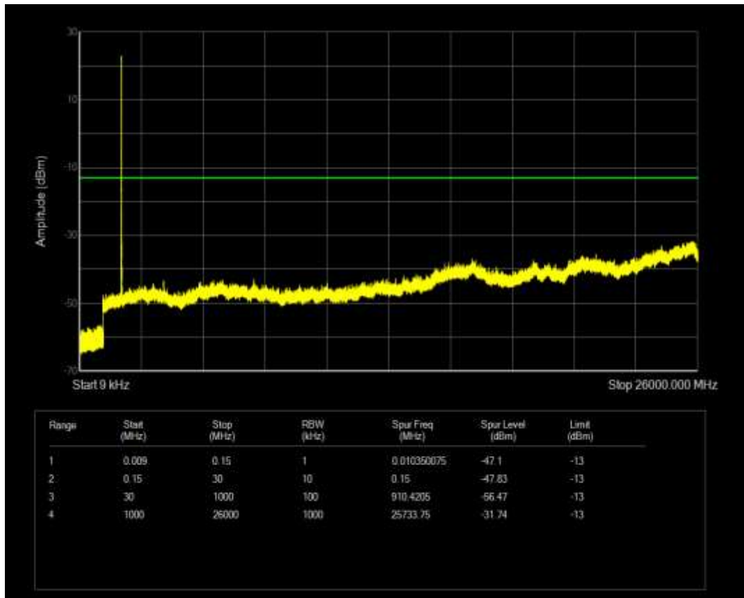
Band66 QPSK BW=10MHz Channel=132622 RB Size=50 Position=#0
