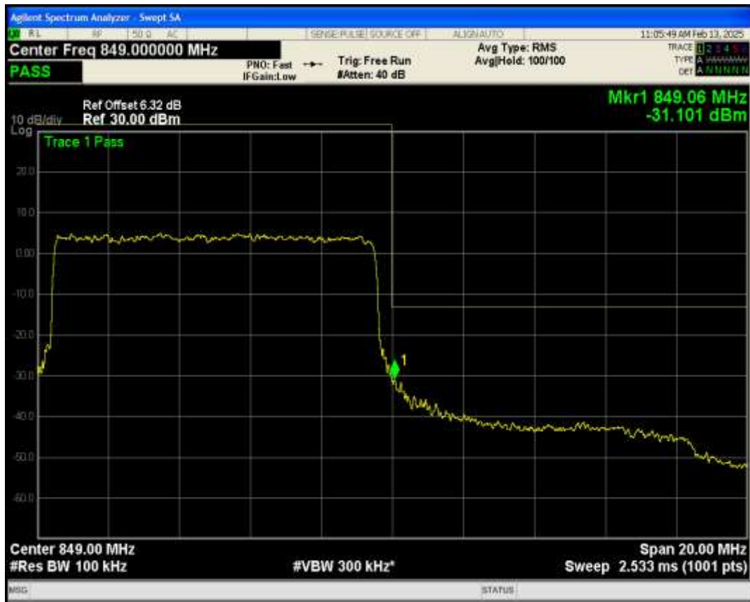
Band66 QPSK BW=1.4MHz Channel=131979 RB Size=6 Position=#0
