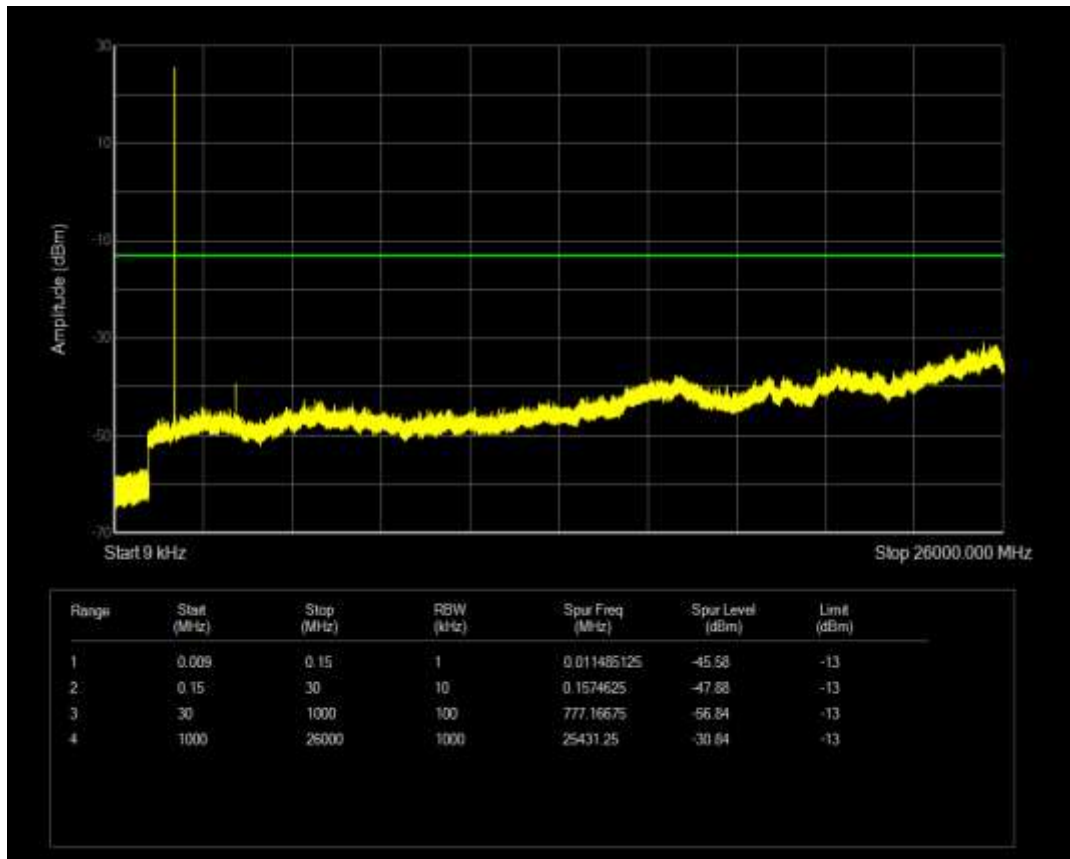
Band66 QPSK BW=3MHz Channel=131987 RB Size=15 Position=#0
