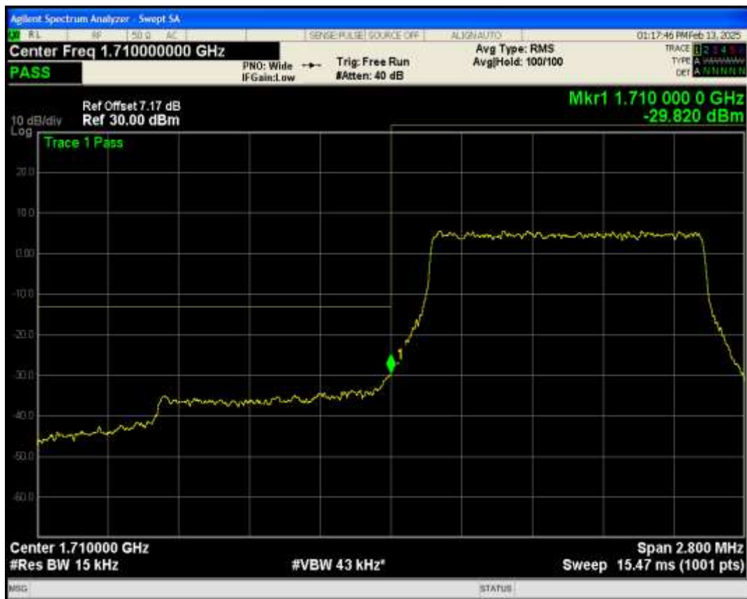
Band66 QAM16 BW=1.4MHz Channel=131979 RB Size=6 Position=#0
