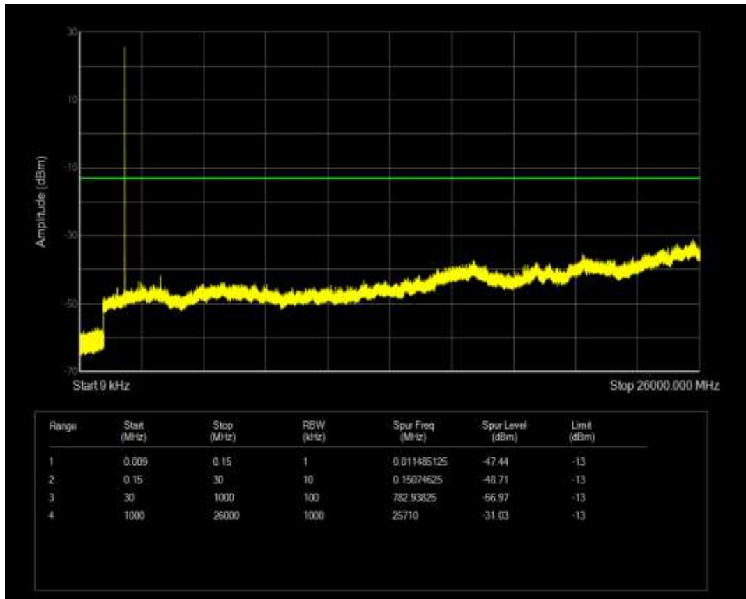
Band2 QPSK BW=3MHz Channel=18615 RB Size=15 Position=#0
