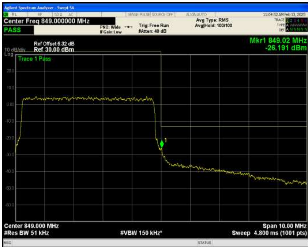
Band5 QPSK BW=10MHz Channel=20600 RB Size=50 Position=#0
