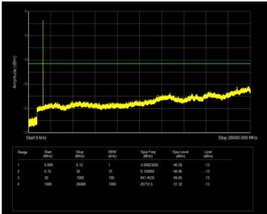
Band4 QAM16 BW=3MHz Channel=20385 RB Size=15 Position=#0
