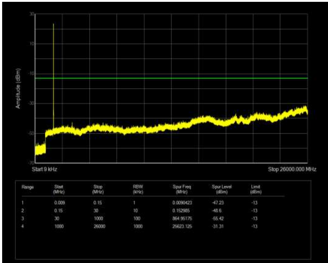
Band66 QAM16 BW=3MHz Channel=131987 RB Size=15 Position=#0
