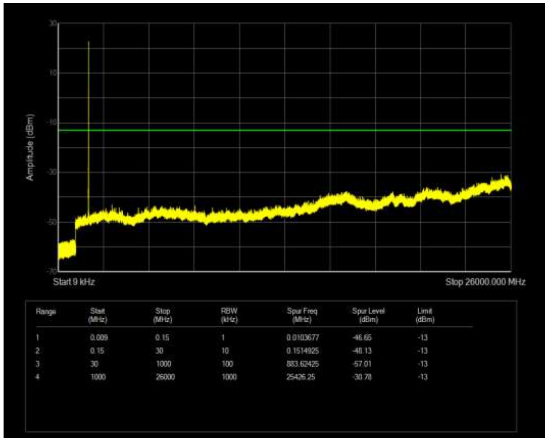
Band4 QPSK BW=5MHz Channel=19975 RB Size=25 Position=#0
