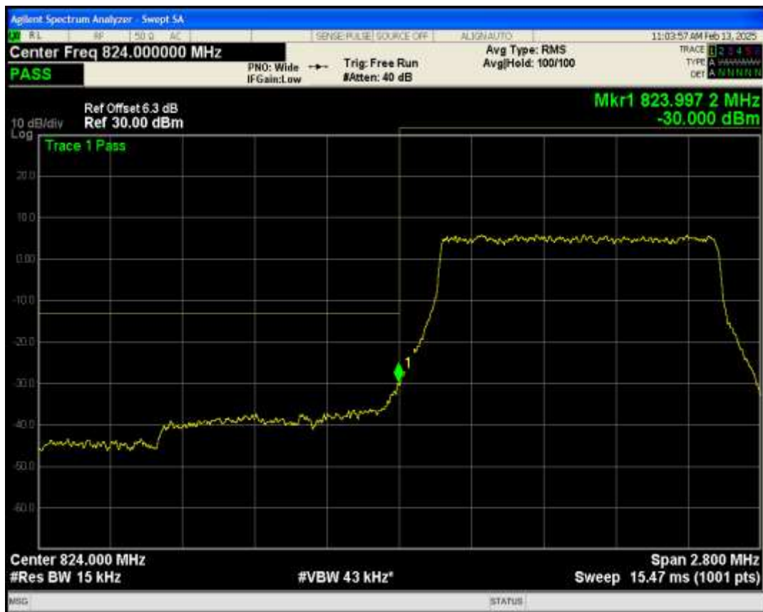
Band5 QAM16 BW=1.4MHz Channel=20407 RB Size=6 Position=#0
