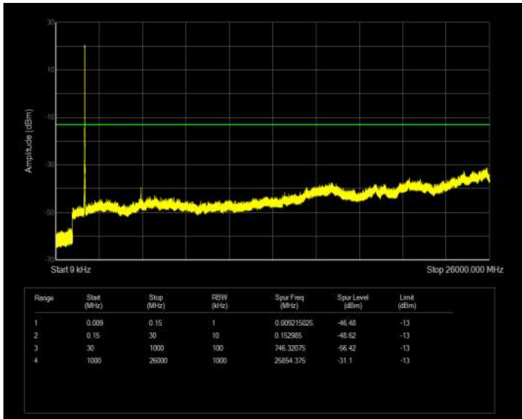
Band4 QPSK BW=15MHz Channel=20025 RB Size=75 Position=#0
