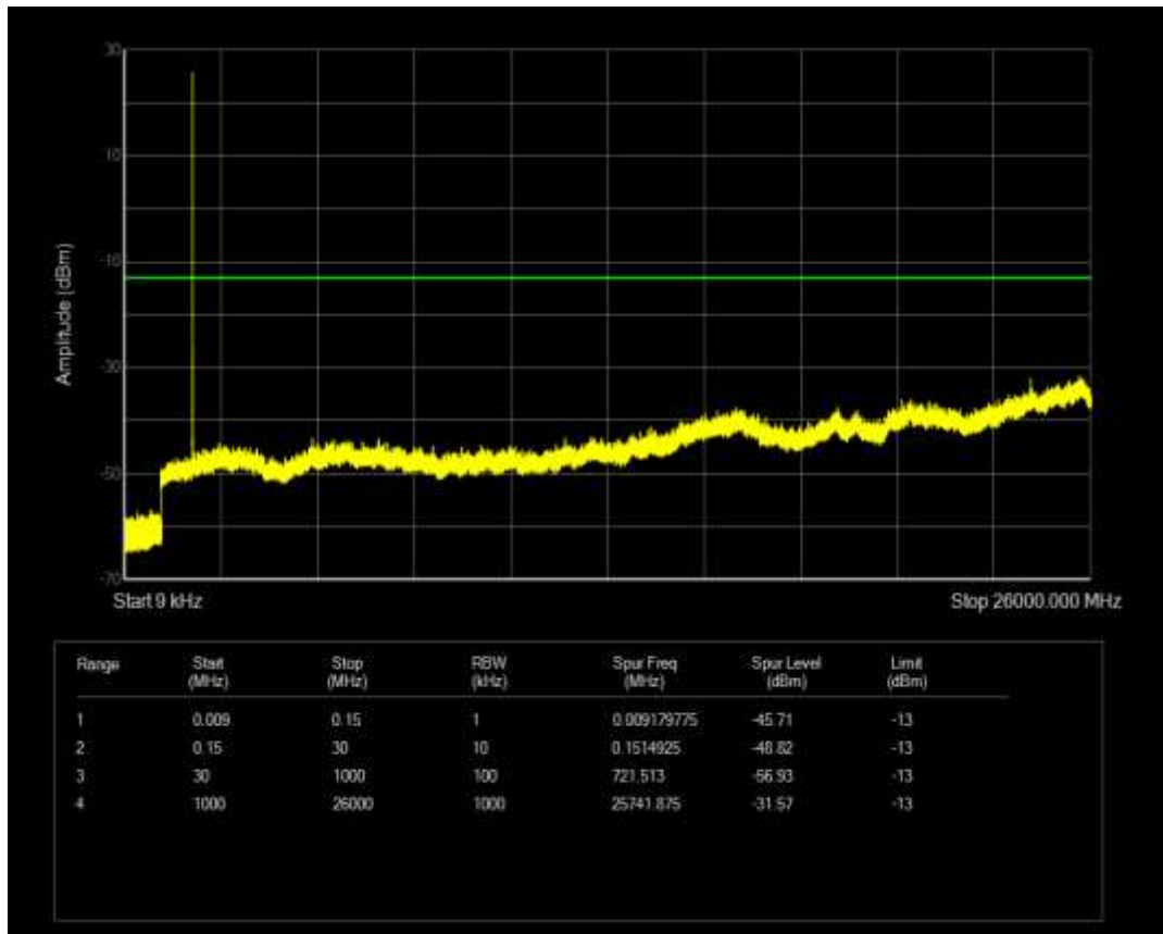
Band2 QAM16 BW=1.4MHz Channel=19193 RB Size=6 Position=#0
