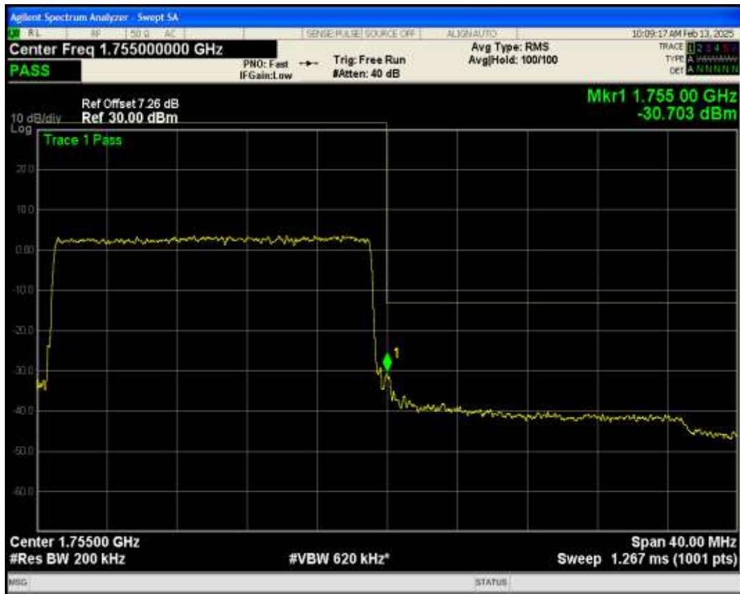
Band5 QPSK BW=1.4MHz Channel=20407 RB Size=6 Position=#0
