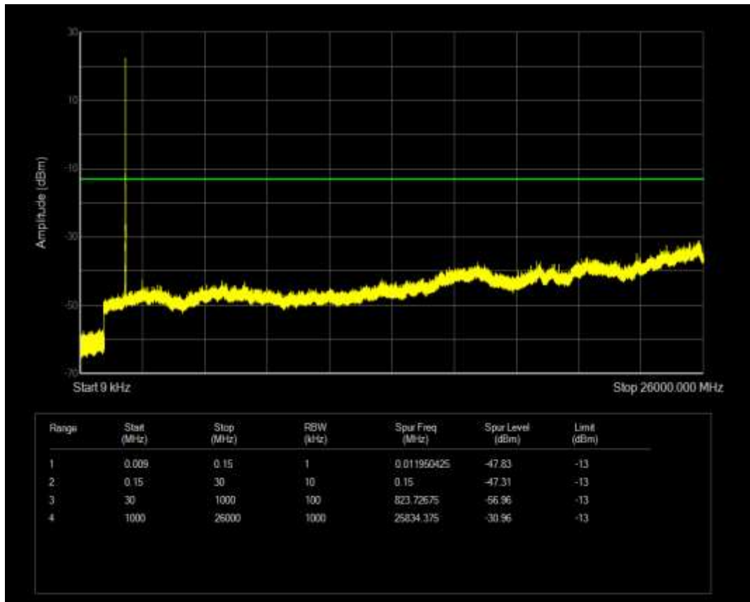
Band2 QAM16 BW=5MHz Channel=18625 RB Size=25 Position=#0
