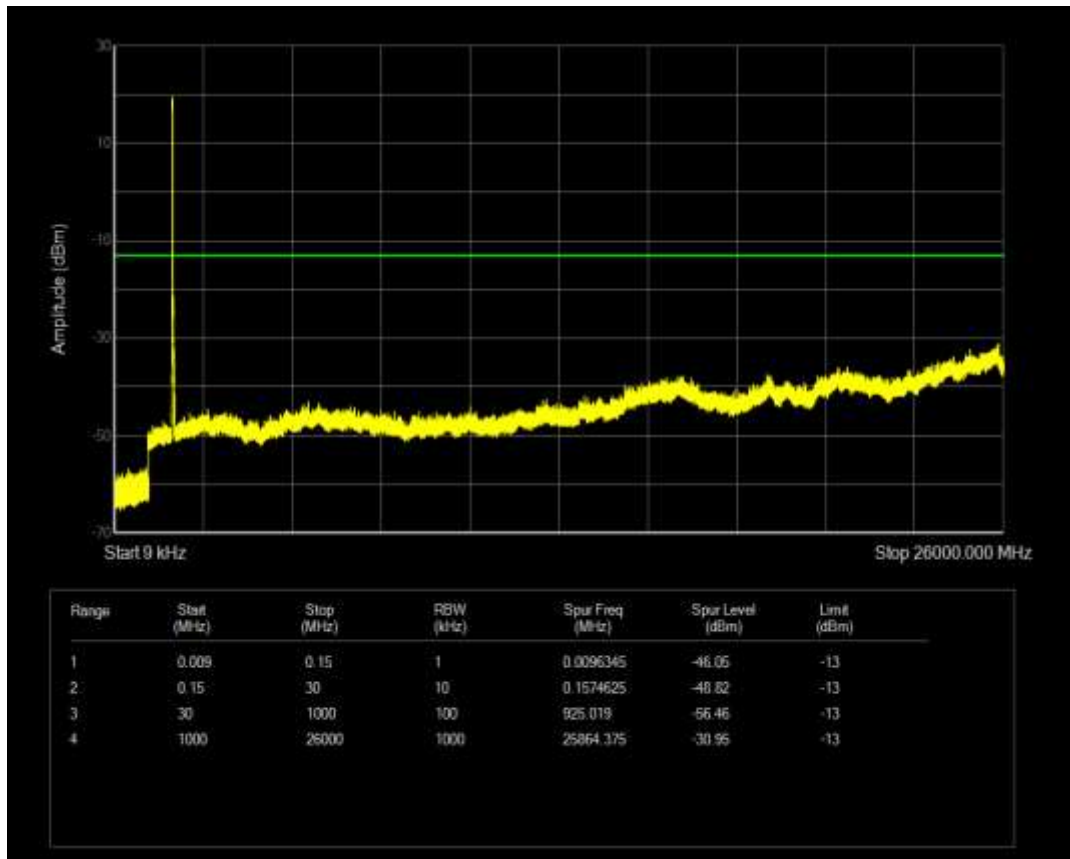
Band66 QPSK BW=20MHz Channel=132072 RB Size=100 Position=#0
