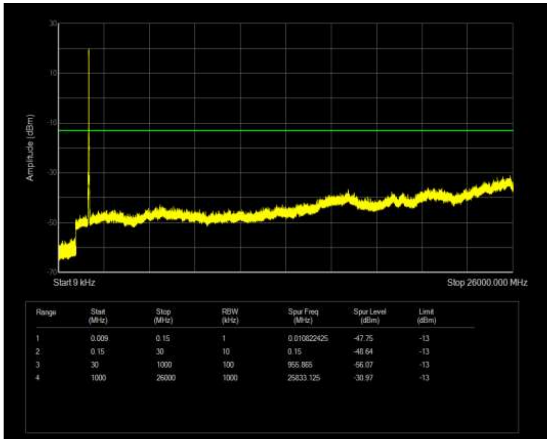
Band4 QPSK BW=20MHz Channel=20050 RB Size=100 Position=#0
