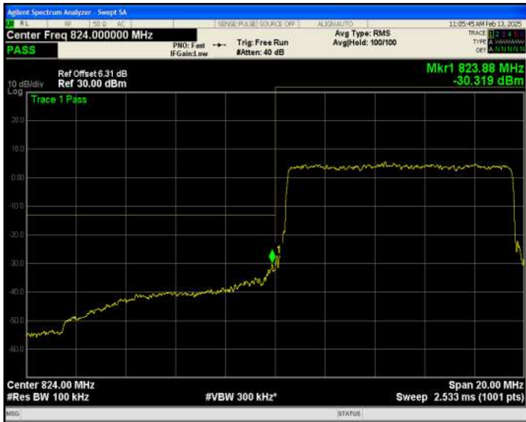
Band5 QAM16 BW=5MHz Channel=20625 RB Size=25 Position=#0
