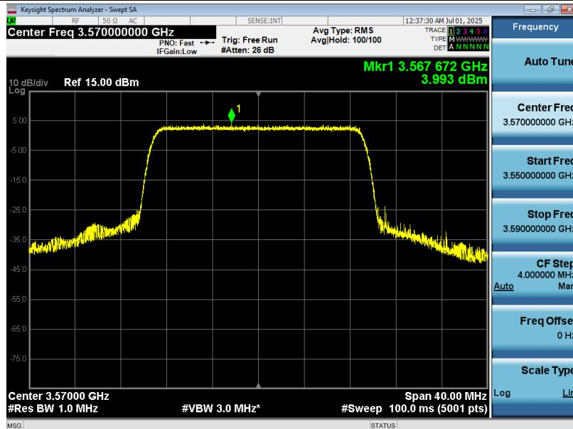
EIRP PSD=3.993-6.12+4.5=2.373dBm/MHz, Antenna gain is -6.12dBi, the path loss is 4.5dB
