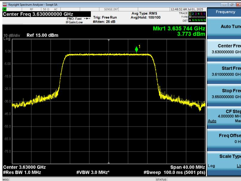
EIRP PSD=3.773-6.12+4.5+3=5.153dBm/MHz, Antenna gain is -6.12dBi, the path loss is 4.5dB, the MIMO Factor is 3dB
