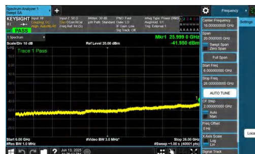
NTNV-n78(3700-3800)-PC2-30-60-L-DFT-BPSK-Inner_1RB_Left-6000 -26000-PASS
