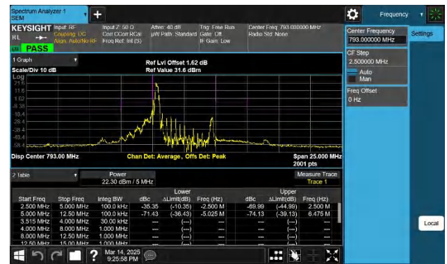
NTNV-Band14-5MHz-16QAM-23330-1RB#0-5.00-12.50-PASS
