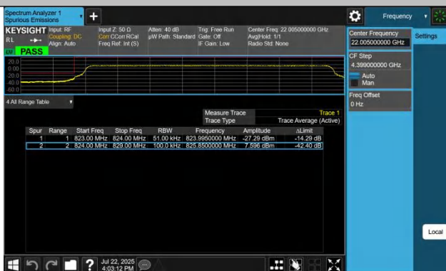
Band5-5MHz-QPSK-20425-25RB#0-PASS
