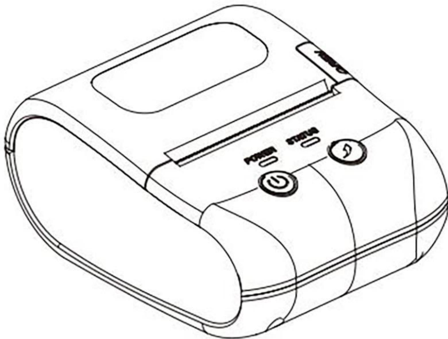
When using the L7 printer (flashing red status light) or L9 printer (paper feed error), please note: Variations in label dimensions, manufacturing processes, materials, or thermal coating thickness across brands/models may cause printer parameter mismatches (head pressure/temperature), leading to printing inaccuracies, jams, or equipment damage.
