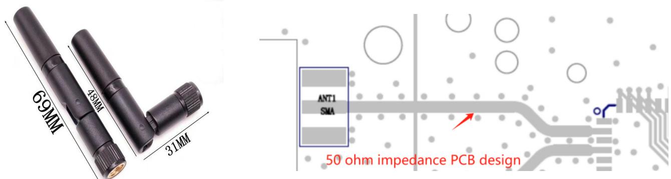
Note: In the PCB layout design part of the antenna, the impedance of the design needs to be strictly modified at 50 ohms. The standard external dual-frequency antenna can be connected through ANT1 SMA, so that the spatial transmission efficiency of the antenna is higher.
