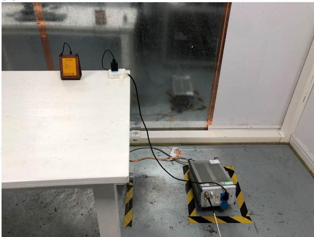
Photo of Power Line Conducted Measurement
