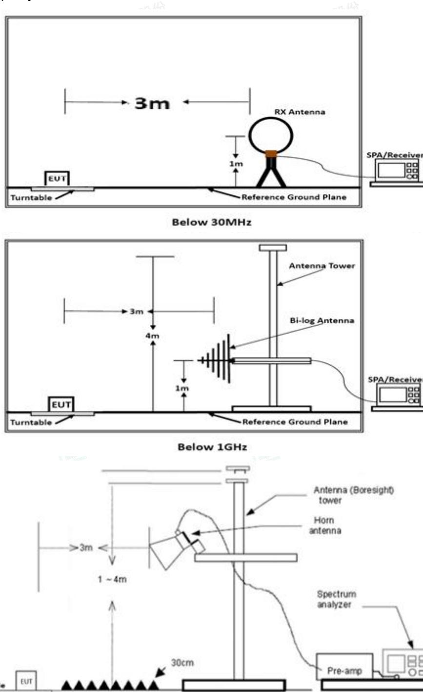
Above 18 GHz shall be extrapolated to the specified distance using an extrapolation factor of 20 dB/decade from 3m to 1m.
