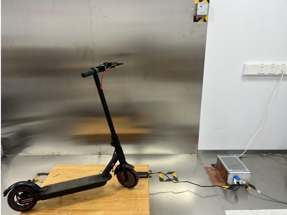
Radiated Emission Test View|(Below 1G)
