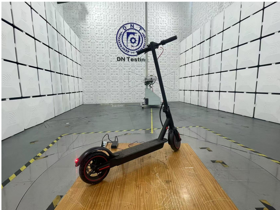
Radiated Emission Test View|(Below 1G)
