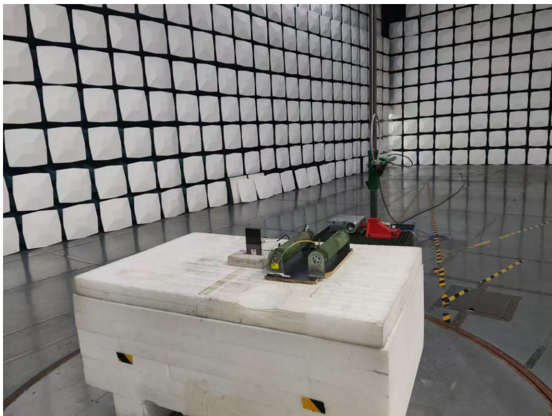
Radiated Emission 9k-30MHz Perpendicular View
