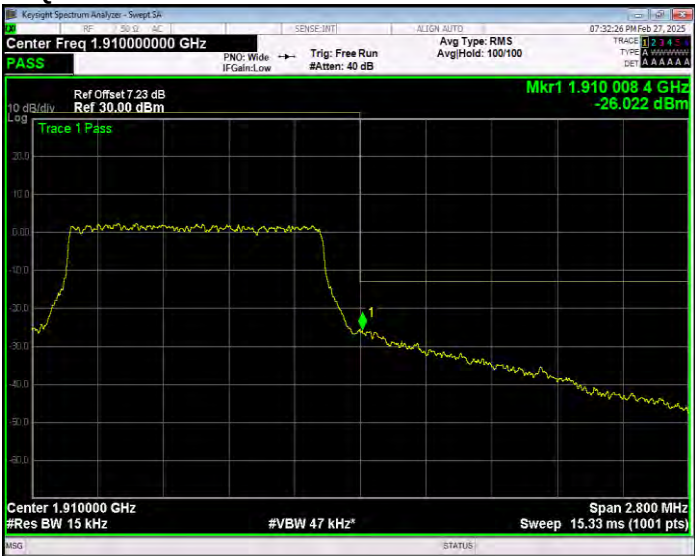
Band2 16QAM BW=1.4MHz Channel=19193 RB Size=6 Position=#0 Normal
