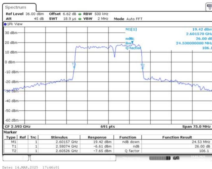
**LTE CA band 41C , 15MHz+10MHz Bandwidth,16QAM (-26dBc BW)**
