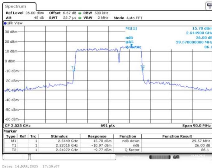
**LTE CA band 7C , 20MHz+10MHz Bandwidth,16QAM (-26dBc BW)**
