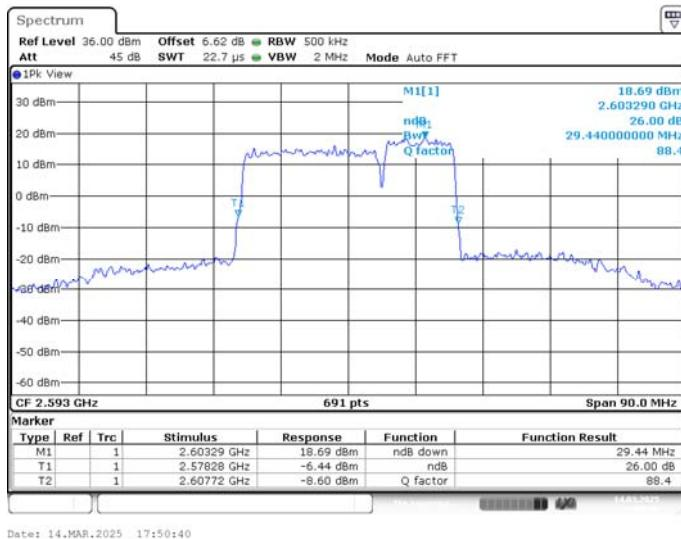
**LTE CA band 41C , 20MHz+10MHz Bandwidth,16QAM (-26dBc BW)**
