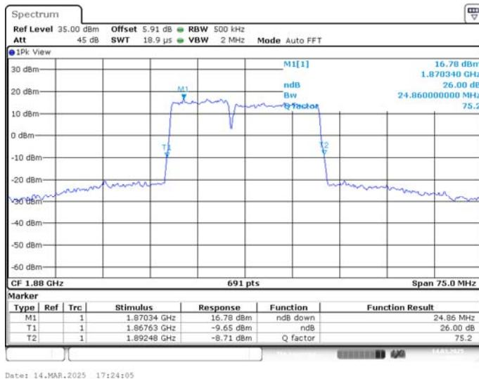
**LTE CA band 2C , 10MHz+15MHz Bandwidth,16QAM (-26dBc BW)**
