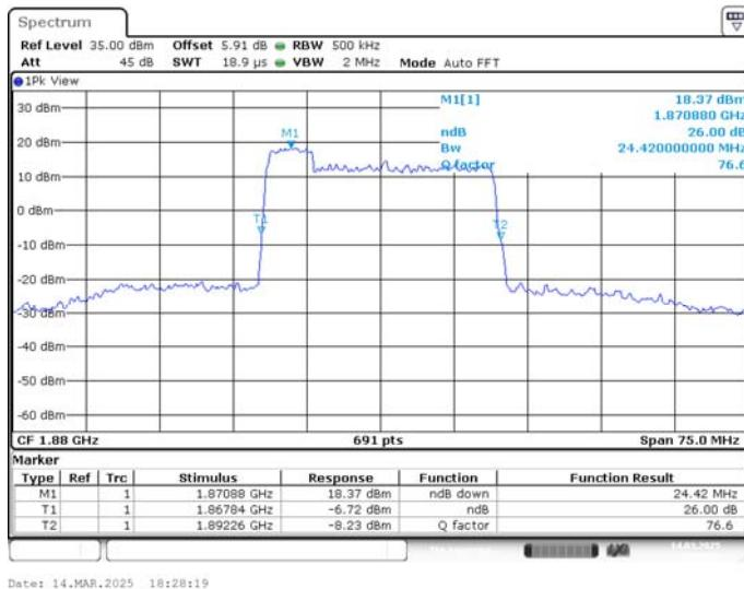
**LTE CA band 2C , 5MHz+20MHz Bandwidth,16QAM (-26dBc BW)**
