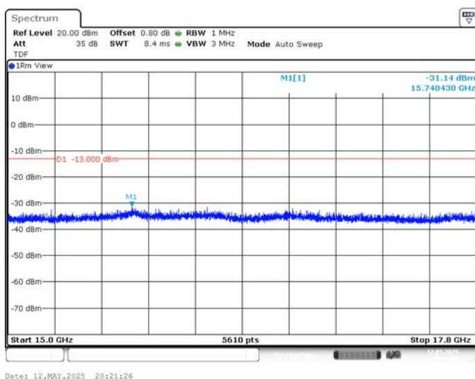
**LTE band 71****NOTE: peak above the limit line is the carrier frequency.**
