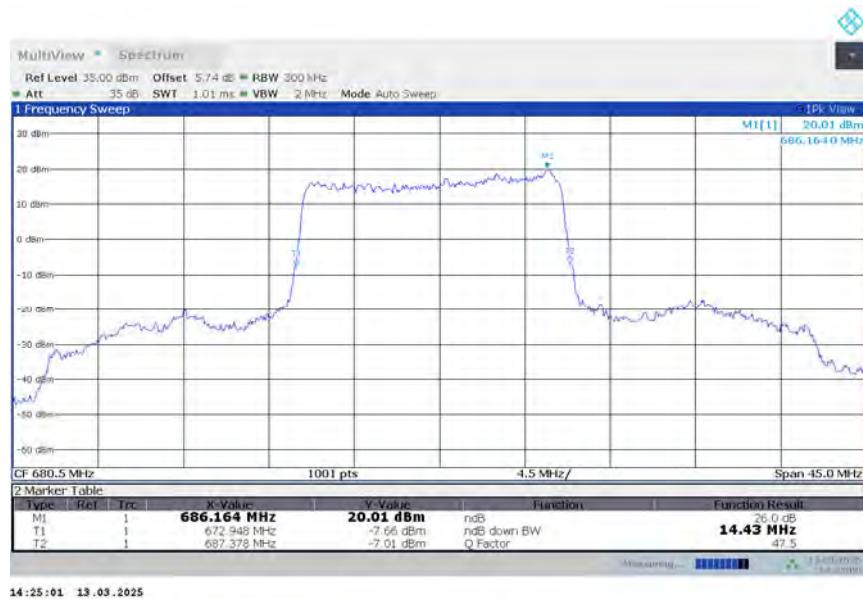
n71,15MHz Bandwidth,DFT-s-QPSK (-26dBc BW)
