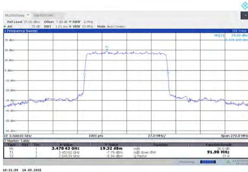
**n78L,90MHz Bandwidth,DFT-s-QPSK (-26dBc BW)**
