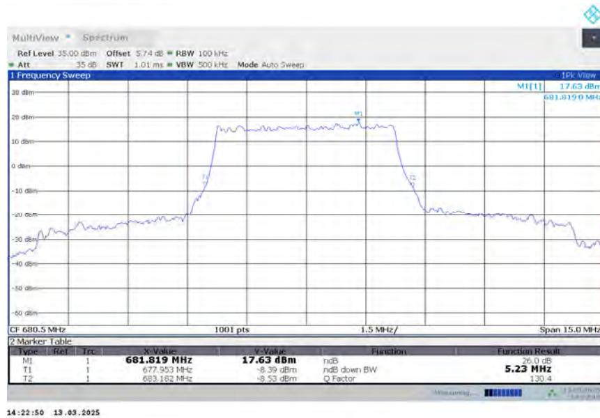
**n71,5MHz Bandwidth,DFT-s-16QAM (-26dBc BW)**
