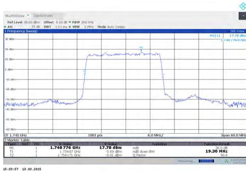
**n66,20MHz Bandwidth,DFT-s-QPSK (-26dBc BW)**
