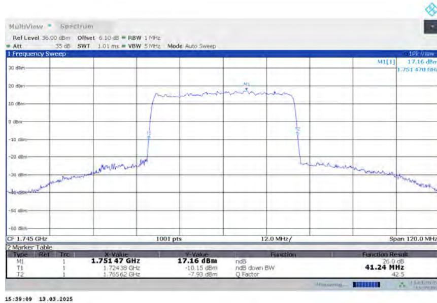
**n66,40MHz Bandwidth,DFT-s-16QAM (-26dBc BW)**
