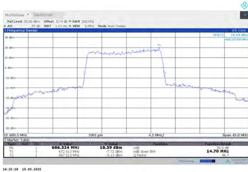
n71,15MHz Bandwidth,DFT-s-16QAM (-26dBc BW)
