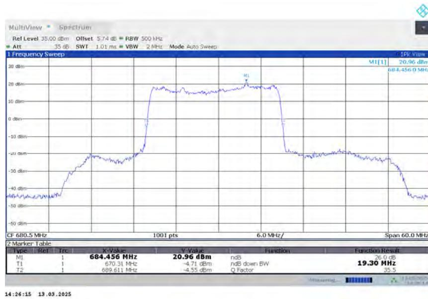
**n71,20MHz Bandwidth,DFT-s-QPSK (-26dBc BW)**
