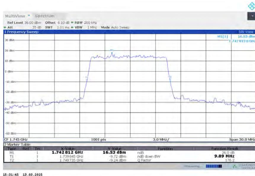
**n66,10MHz Bandwidth,DFT-s-16QAM (-26dBc BW)**
