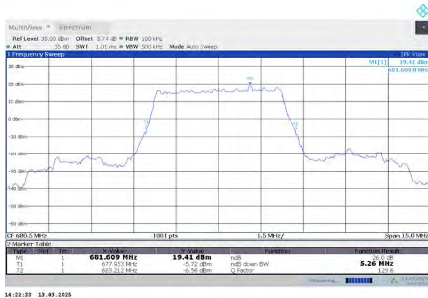
**n71,5MHz Bandwidth,DFT-s-QPSK (-26dBc BW)**
