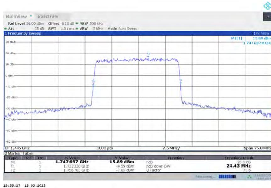
**n66,25MHz Bandwidth,DFT-s-16QAM (-26dBc BW)**
