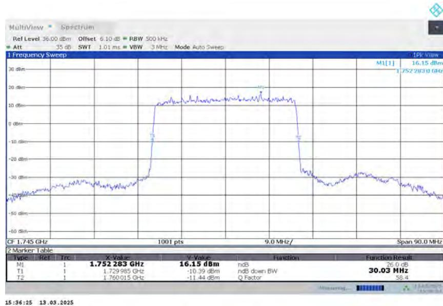
**n66,30MHz Bandwidth,DFT-s-QPSK (-26dBc BW)**
