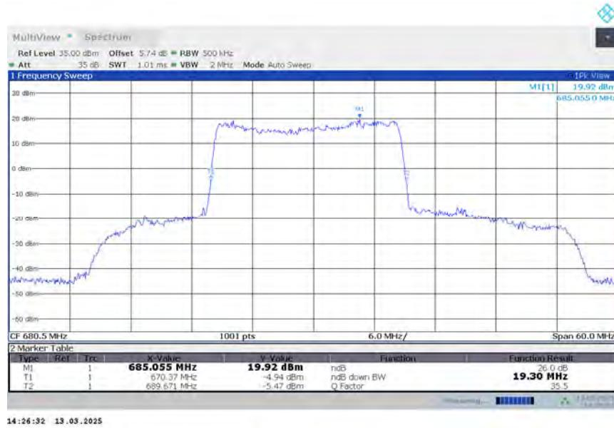
**n71,20MHz Bandwidth,DFT-s-16QAM (-26dBc BW)**
