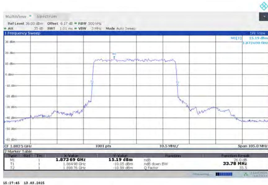
**n25,35MHz Bandwidth,DFT-s-QPSK (-26dBc BW)**
