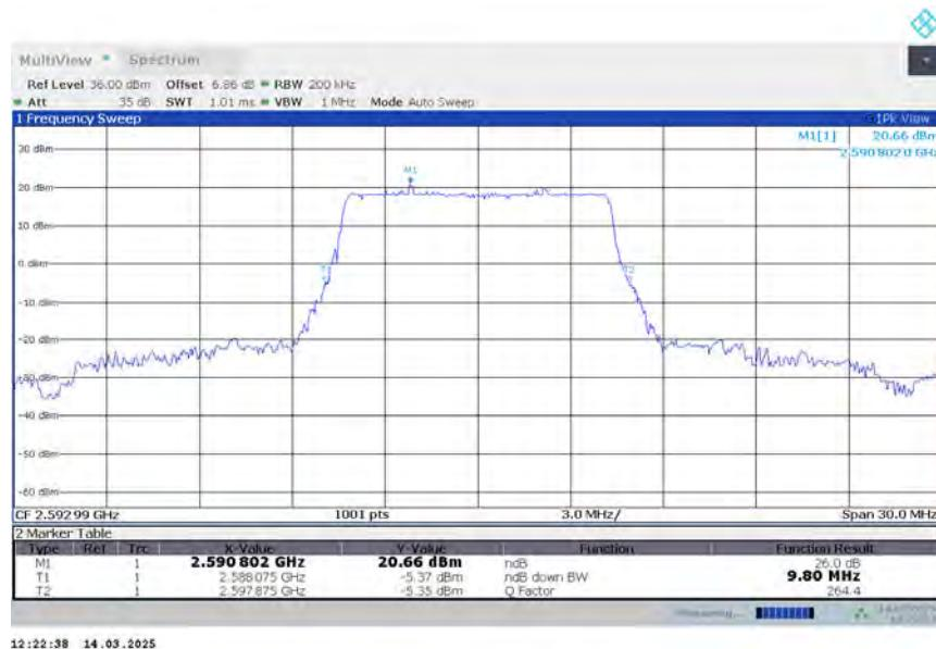
**n41,10MHz Bandwidth,DFT-s-QPSK (-26dBc BW)**
