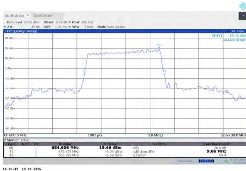
**n71,10MHz Bandwidth,DFT-s-QPSK (-26dBc BW)**
