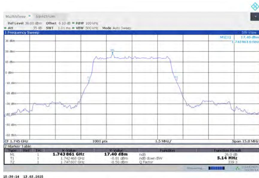
**n66,5MHz Bandwidth,DFT-s-QPSK (-26dBc BW)**
