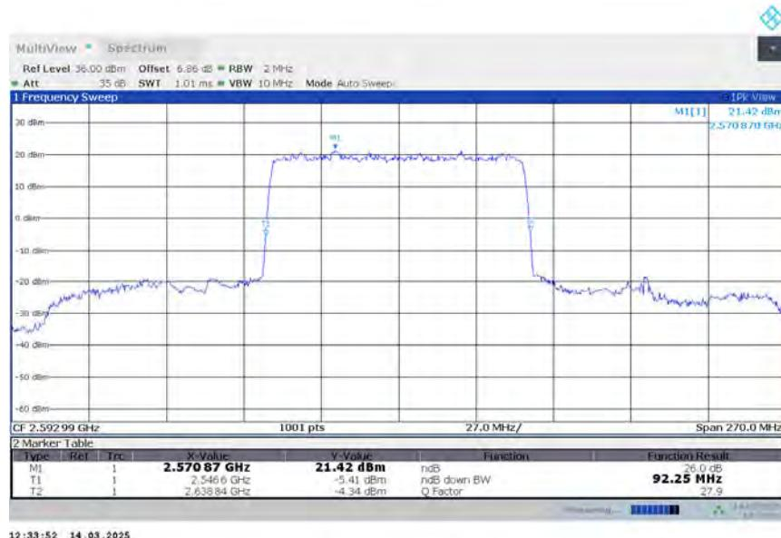
**n41,90MHz Bandwidth,DFT-s-QPSK (-26dBc BW)**
