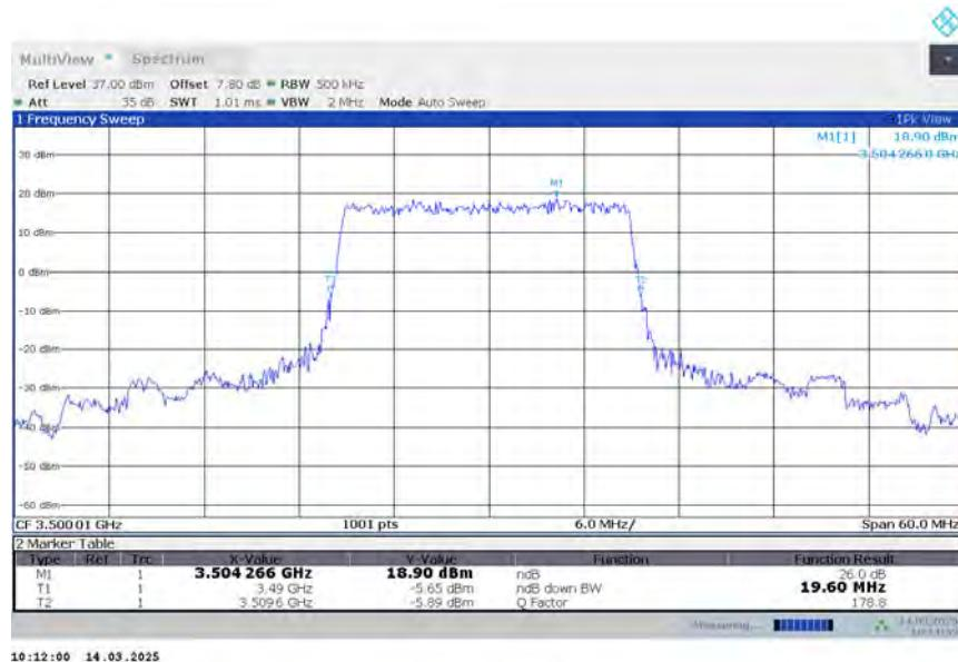
**n78L,20MHz Bandwidth,DFT-s-QPSK (-26dBc BW)**
