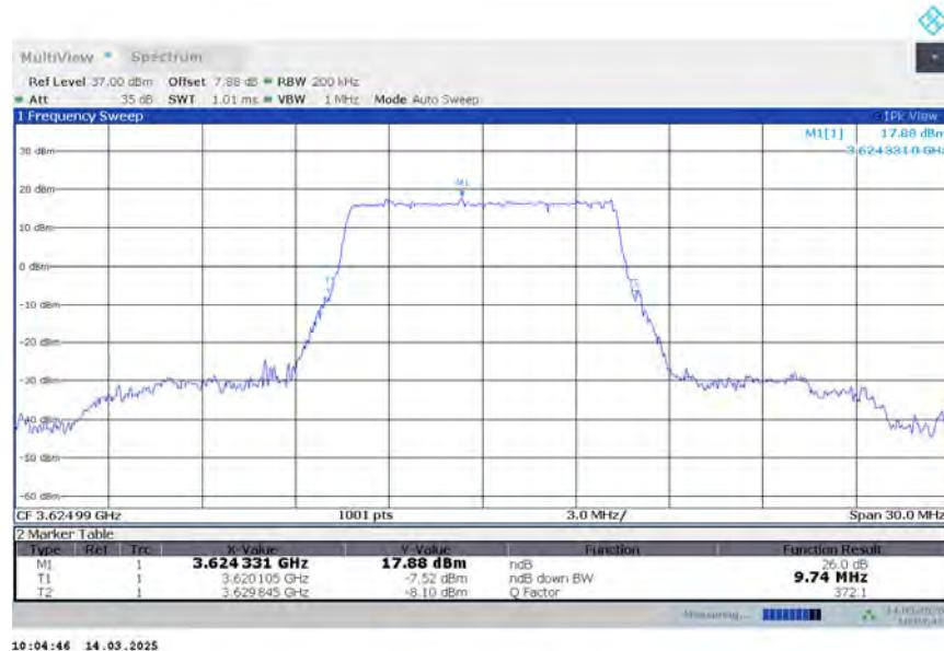
**n48,10MHz Bandwidth,DFT-s-16QAM (-26dBc BW)**
