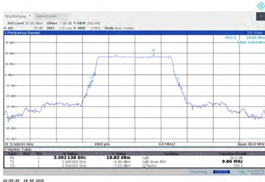
**n78L,10MHz Bandwidth,DFT-s-QPSK (-26dBc BW)**
