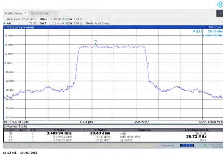
**n78L,40MHz Bandwidth,DFT-s-QPSK (-26dBc BW)**
