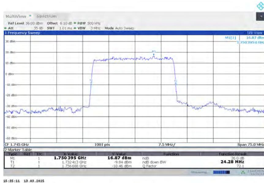
**n66,25MHz Bandwidth,DFT-s-QPSK (-26dBc BW)**
