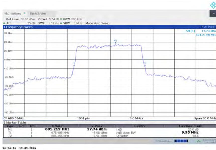
**n71,10MHz Bandwidth,DFT-s-16QAM (-26dBc BW)**
