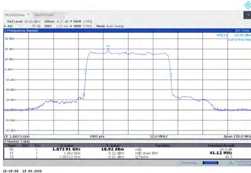
**n25,40MHz Bandwidth,DFT-s-QPSK (-26dBc BW)**
