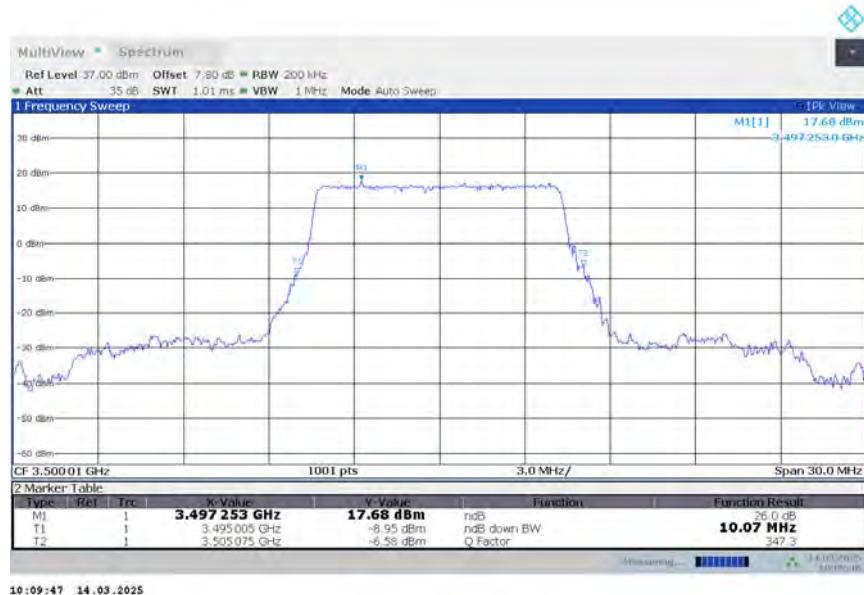
**n78L,10MHz Bandwidth,DFT-s-16QAM (-26dBc BW)**
