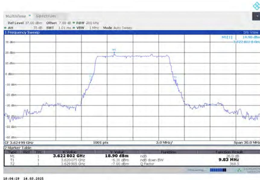
**n48,10MHz Bandwidth,DFT-s-QPSK (-26dBc BW)**
