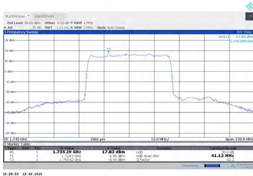
**n66,40MHz Bandwidth,DFT-s-QPSK (-26dBc BW)**
