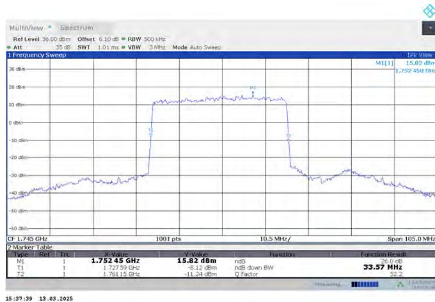
**n66,35MHz Bandwidth,DFT-s-QPSK (-26dBc BW)**
