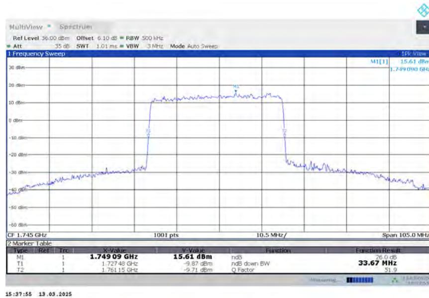
**n66,35MHz Bandwidth,DFT-s-16QAM (-26dBc BW)**
