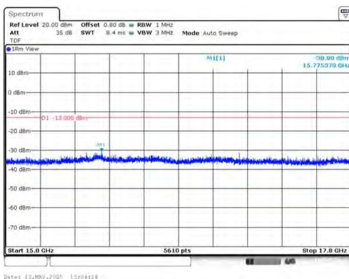
**LTE band 71****NOTE: peak above the limit line is the carrier frequency.**
