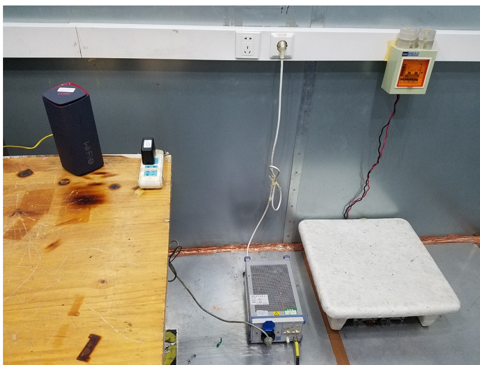
Picture 2 Conducted Emission Test Setup
