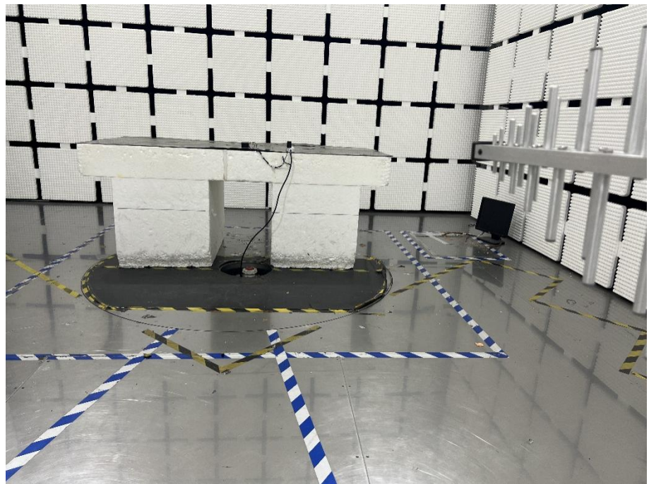
Radiation Emission Test Setup (30MHz to 1GHz)
