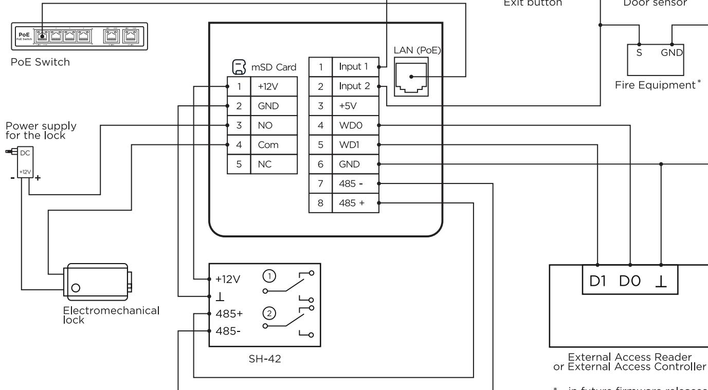
Connection scheme of electromagnetic lock using PoE for panel and additional power supply for the lock
