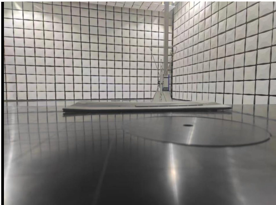
Radiated Emissions Test Setup (30-1000MHz)
