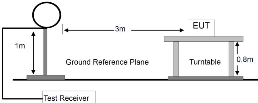
For Radiated Emission 30-1000MHz
