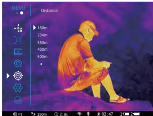
Each configuration table can save up to 6 different distance values. After selecting a distance value, enter the adjustment interface. Select “+” to increase the zero calibration distance value.
