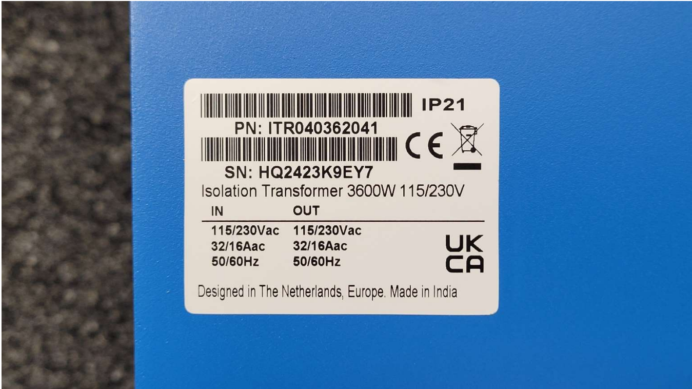
Photo No. 43: AC/AC converter/transformer 115 / 230 V AC used for testing
