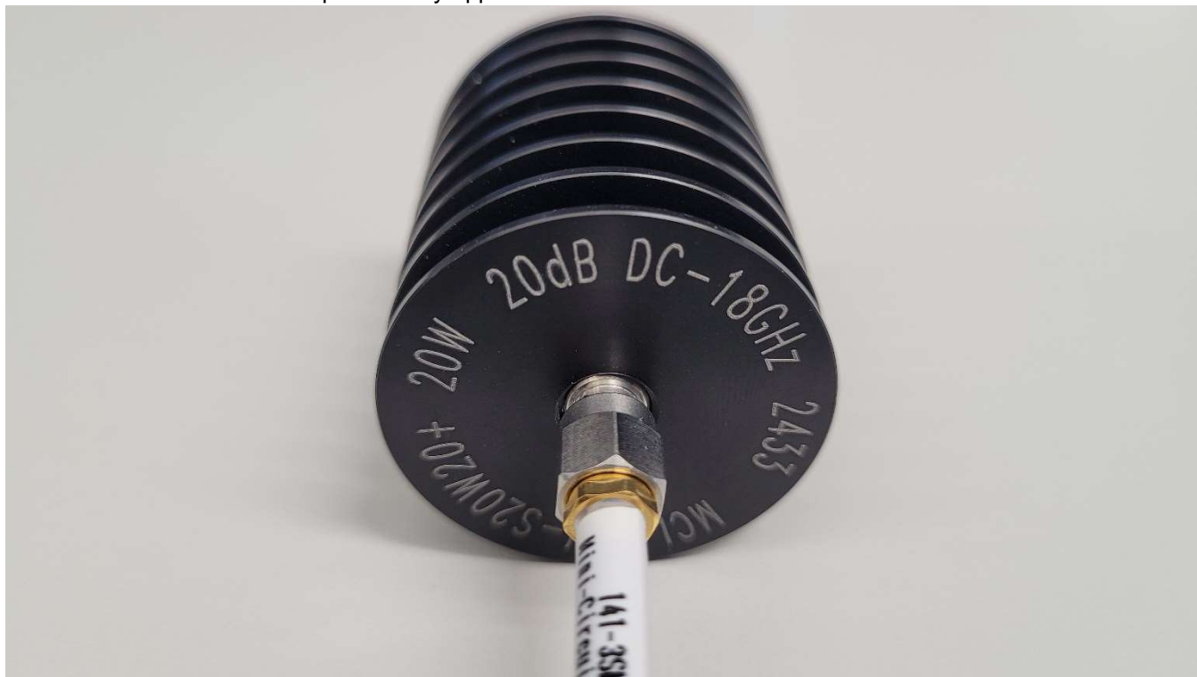
Photo No. 40: attenuator/load provided by applicant
