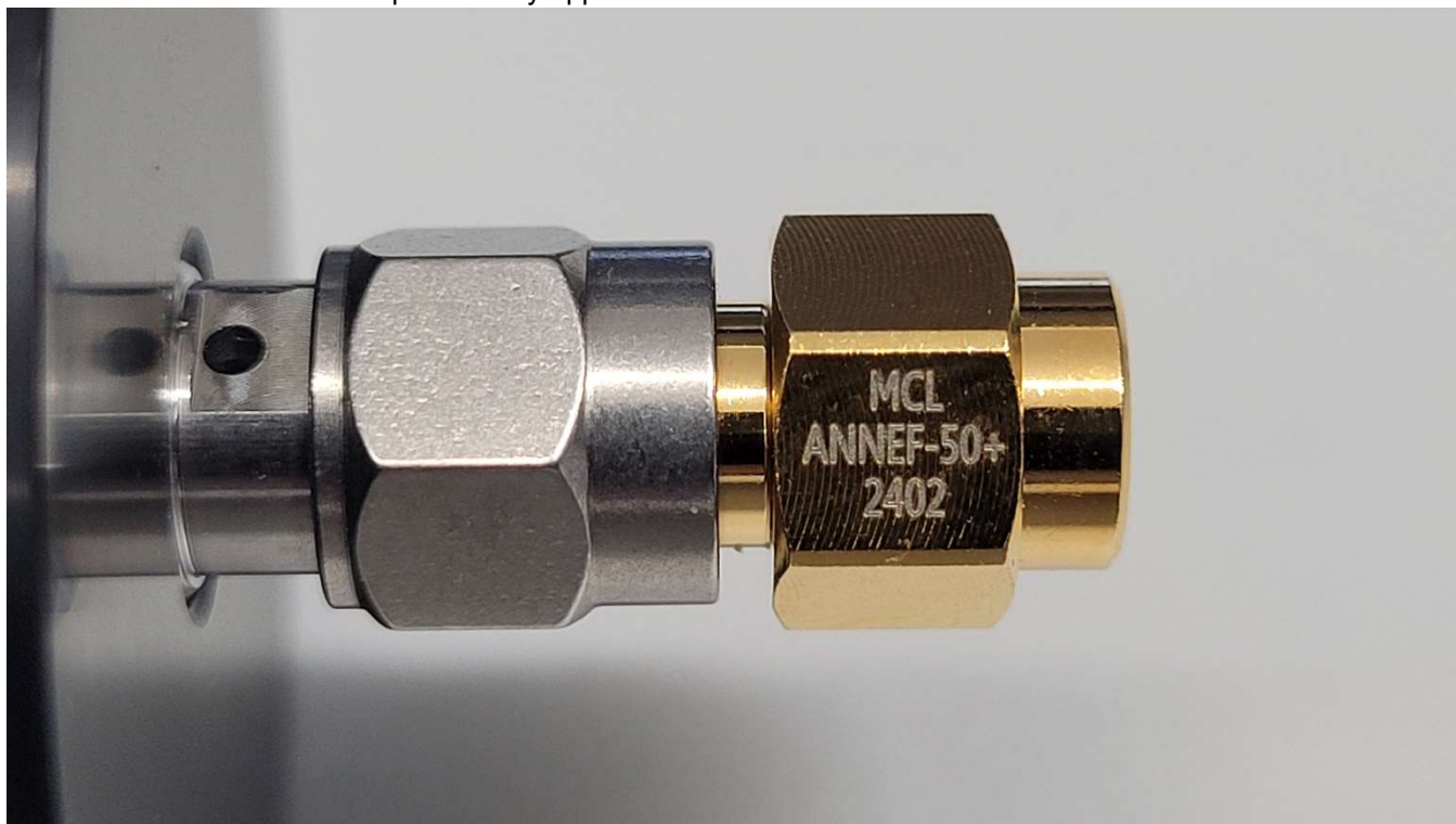
Photo No. 41: attenuator/load provided by applicant
