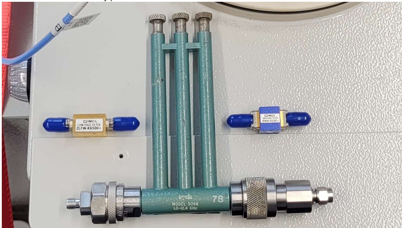
Photo No. 36: filters externally provided
