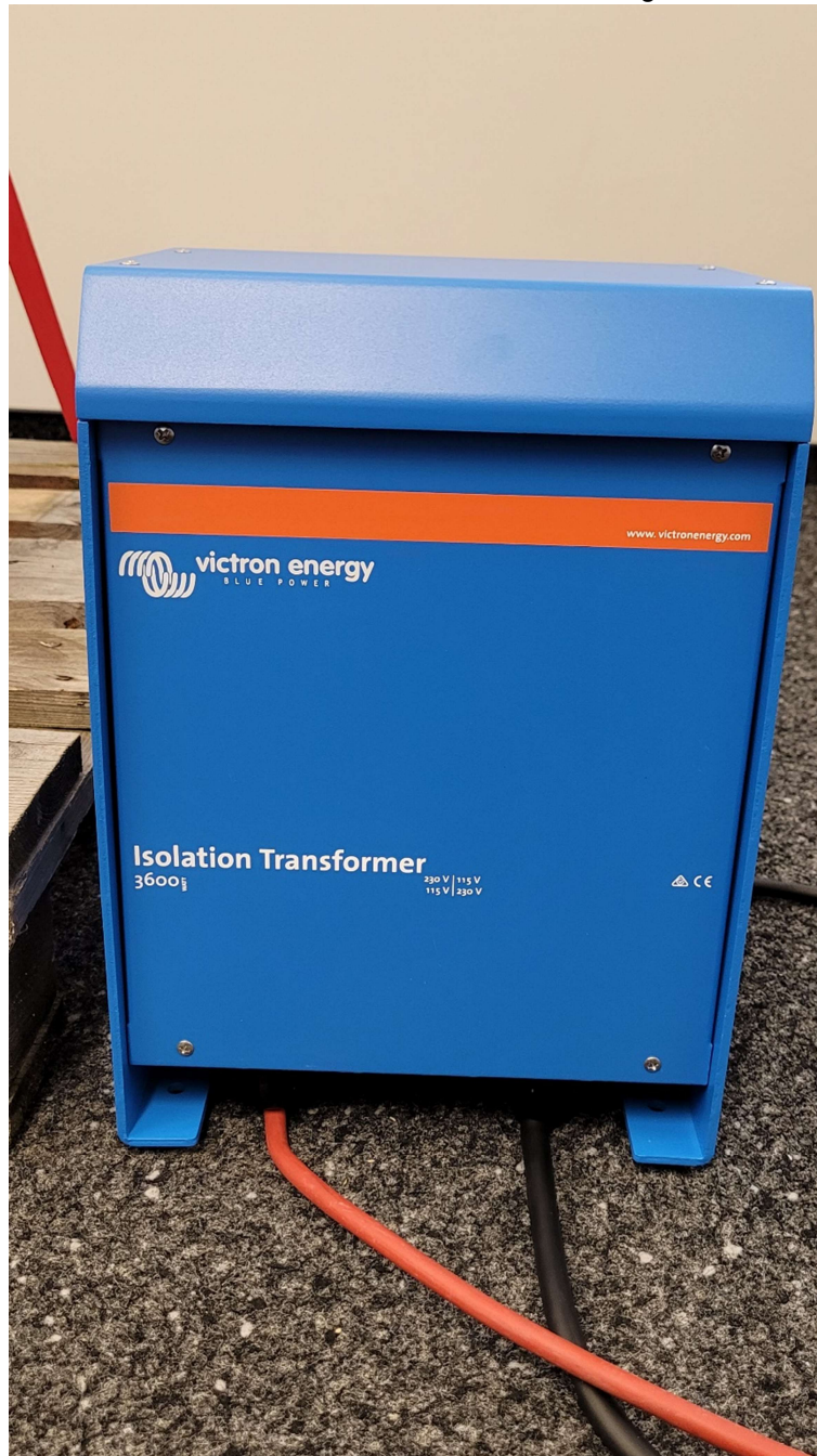
Photo No. 42: AC/AC converter/transformer 115 / 230 V AC used for testing
