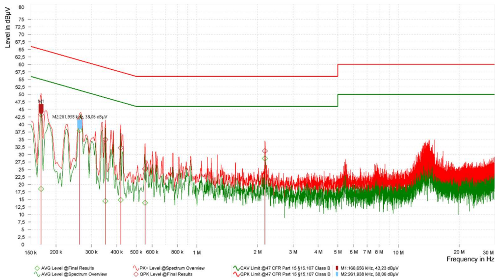
Plot no. 26: conducted emissions, line L1, CH1
