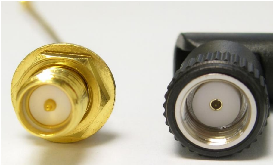
Dipole Antenna to Cable Connection
