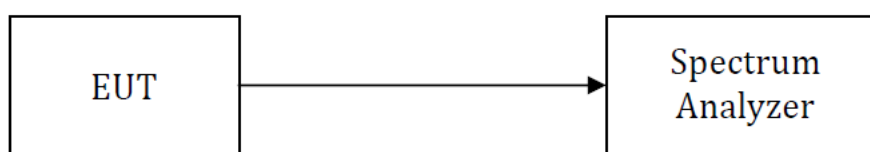
Test Setup Block Diagram
