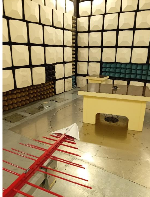
Test Setup – AC Power Line Conducted Emissions
