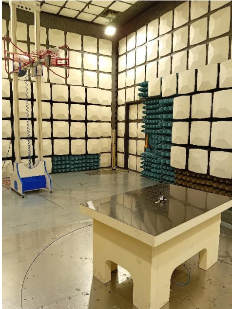
Test Setup – AC Power Line Conducted Emissions
