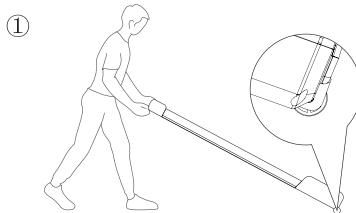
01. Place the machine on a level surface with a gap of 19.7 inches/0.5m in front and back.
