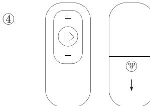
04. Make sure the batteries are properly installed in the back of the remote controller, then press the "On/Off" key.
