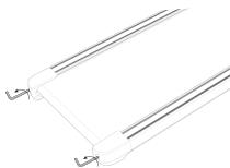
02. When the running belt is too tight, it will cause stronger resistance. Please turn the screws on both sides counterclockwise 1-2 turns: Loosen the belt until it stops slipping or pausing; when the running belt is too loose, please turn the screws on both sides clockwise 1-2 turns.
