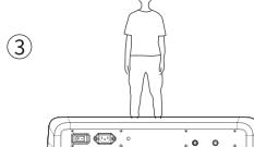
(3). Start the treadmill and lubricate for 10-20 seconds at a speed of 3mph/4.8kph.
