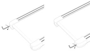
01. When the running belt is tilted to the left, adjust the screw 1-2 turns clockwise to the left. When the running belt tilts to the right, adjust the screw 1-2 turns clockwise to the right. Then, test run; if the running belt is still tilted, repeat the above steps until the running belt is aligned.
