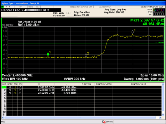
Out Of Band Emission(Left) 8DPSK_3-DH5_Channel Hopping
