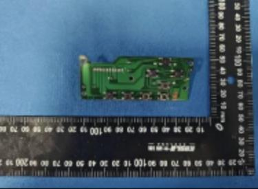
A photograph of the green keyboard PCB for the 82104 model. It is placed on a blue surface next to a metric ruler.  |
