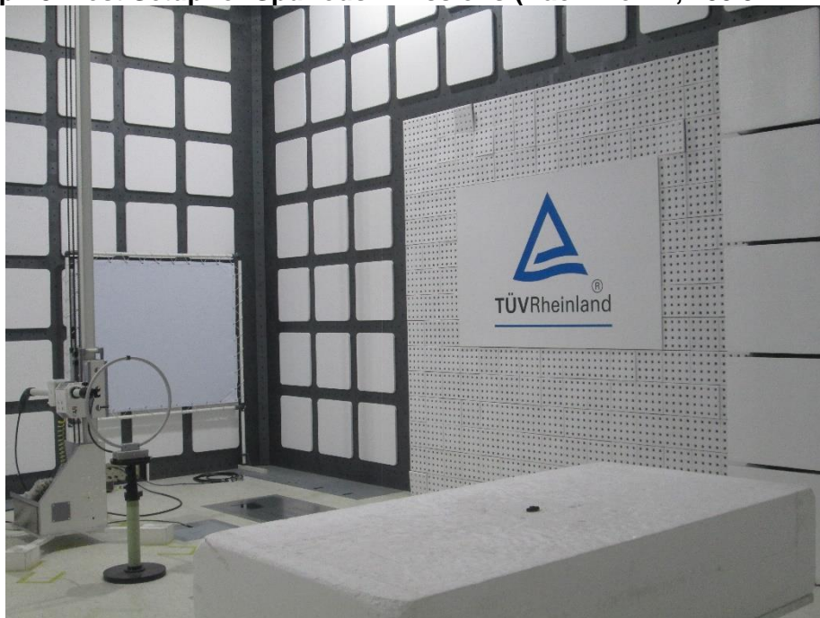
Photograph 8: Test Setup for Spurious Emissions (Back View 1, 433.92MHz)
