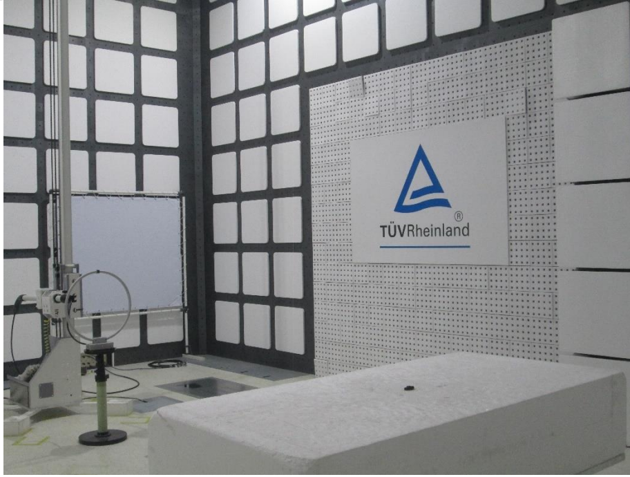
Photograph 4: Test Setup for Spurious Emissions (Back View 2, 315MHz)
