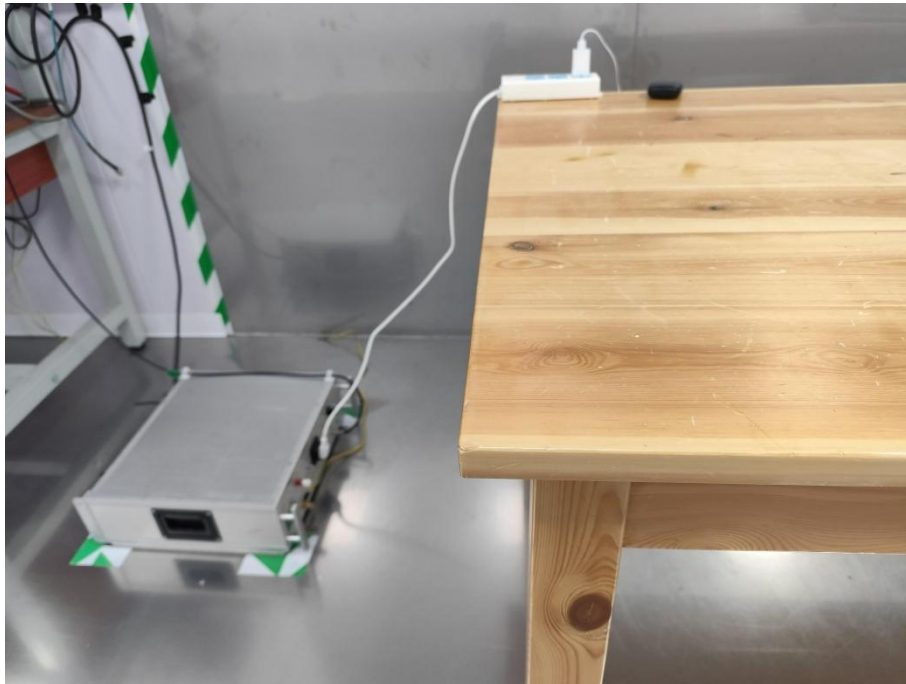
Conducted Emission at AC power line
