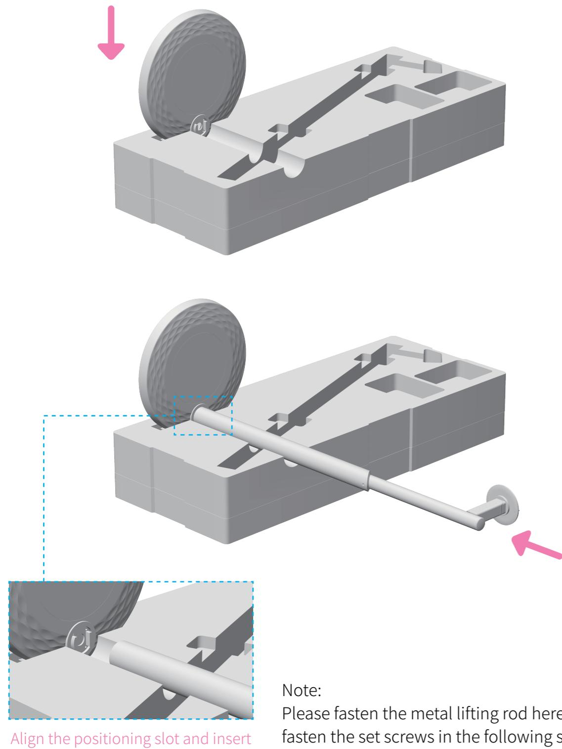
Align the positioning slot and insert
