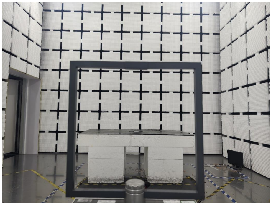
Radiation Emission Test Setup (Below 30MHz)
