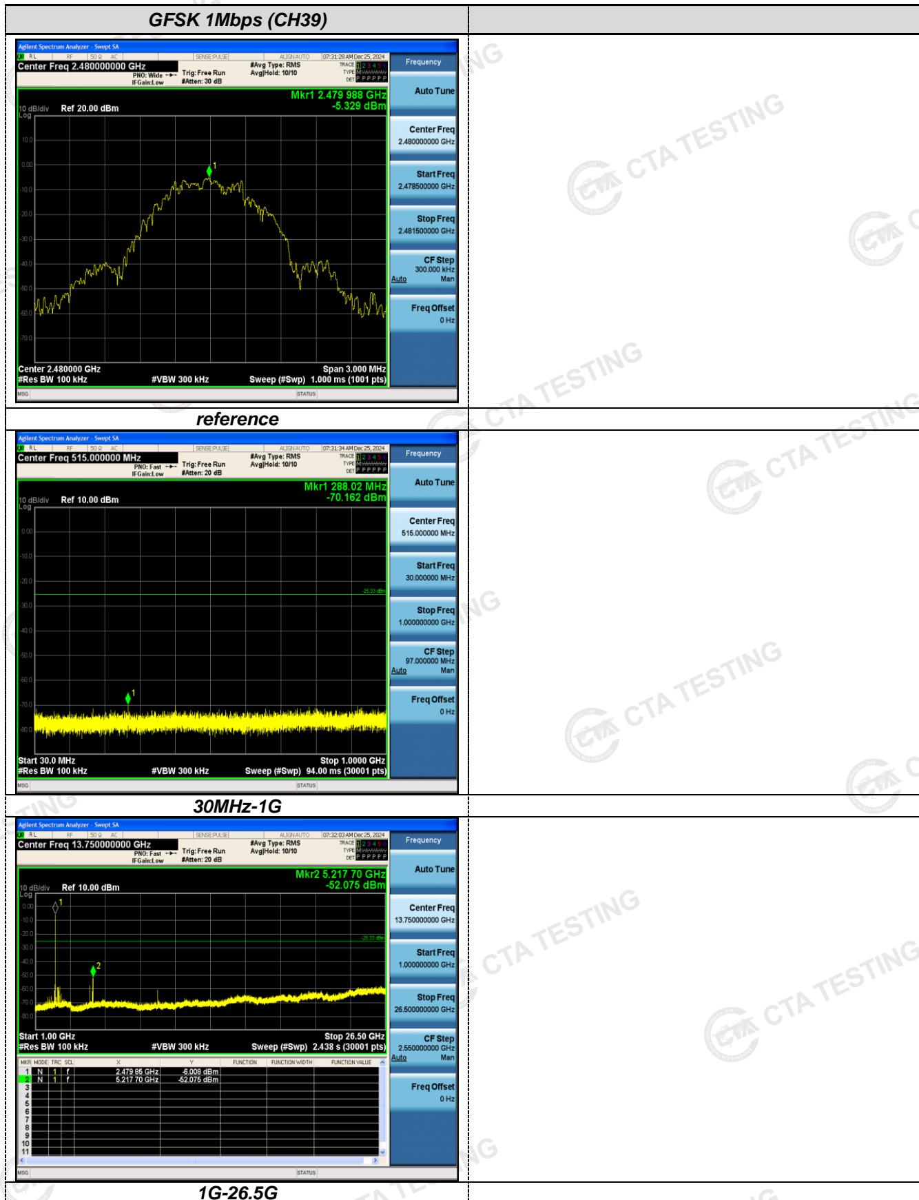
Band-edge Measurements for RF Conducted Emissions:
