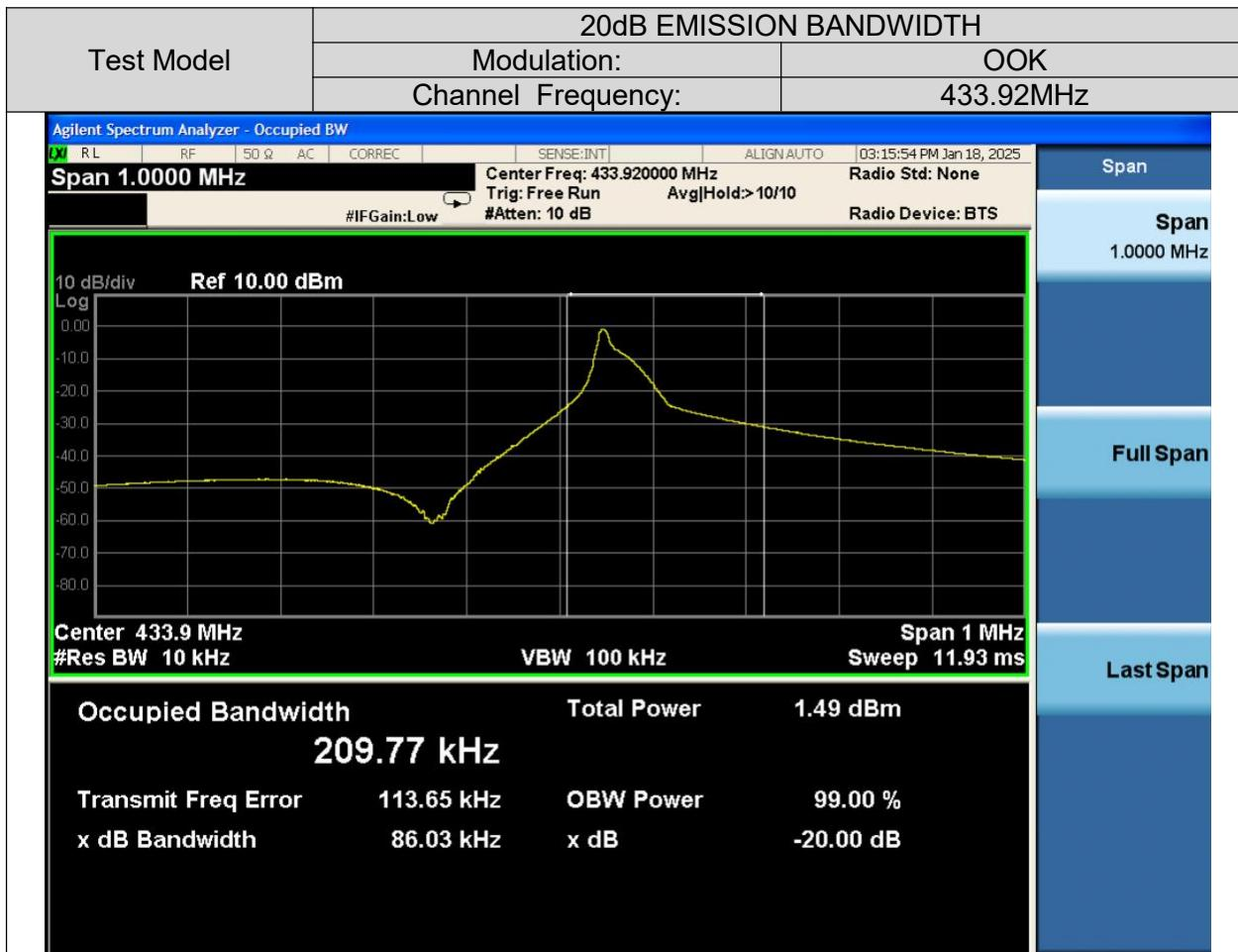
Note: The resolution bandwidth (RBW) shall be in the range of 1% to 5% of the occupied bandwidth (OBW) and video bandwidth (VBW) shall be approximately 3x RBW.
